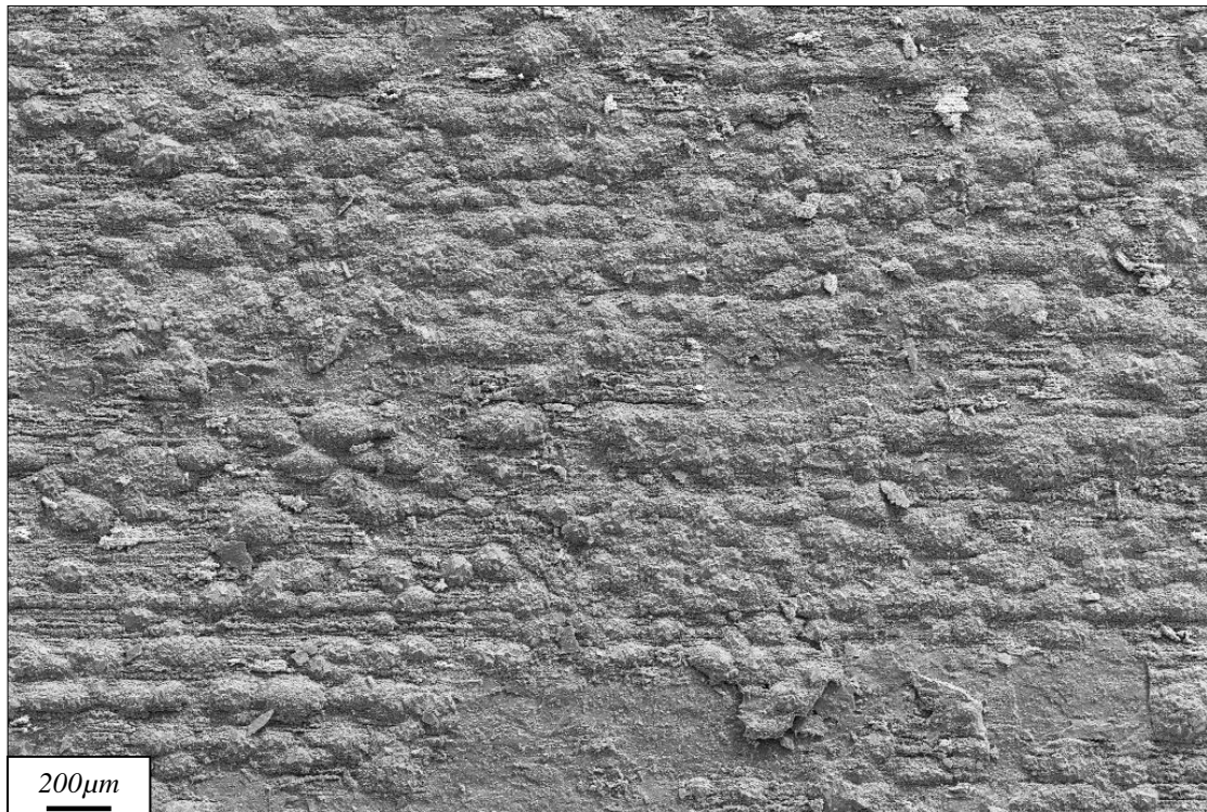
Figure 9.5: Secondary electron images of the surface oxide formed on industrially ground S32101 after simulated reheat to a final temperature of 1220°C in the experimental reheat furnace
