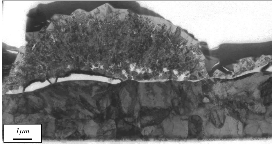
Figure 8.27:- Bright field transmission electron micrograph of a cross-section of an oxide nodule formed on industrially ground S32205 after oxidation at 1000°C for 1 hour in simulated propane combustion products
