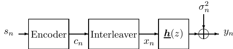
Figure 4.6: Transmitter section of the SBR2 system forming a serial concatenated encoder.
