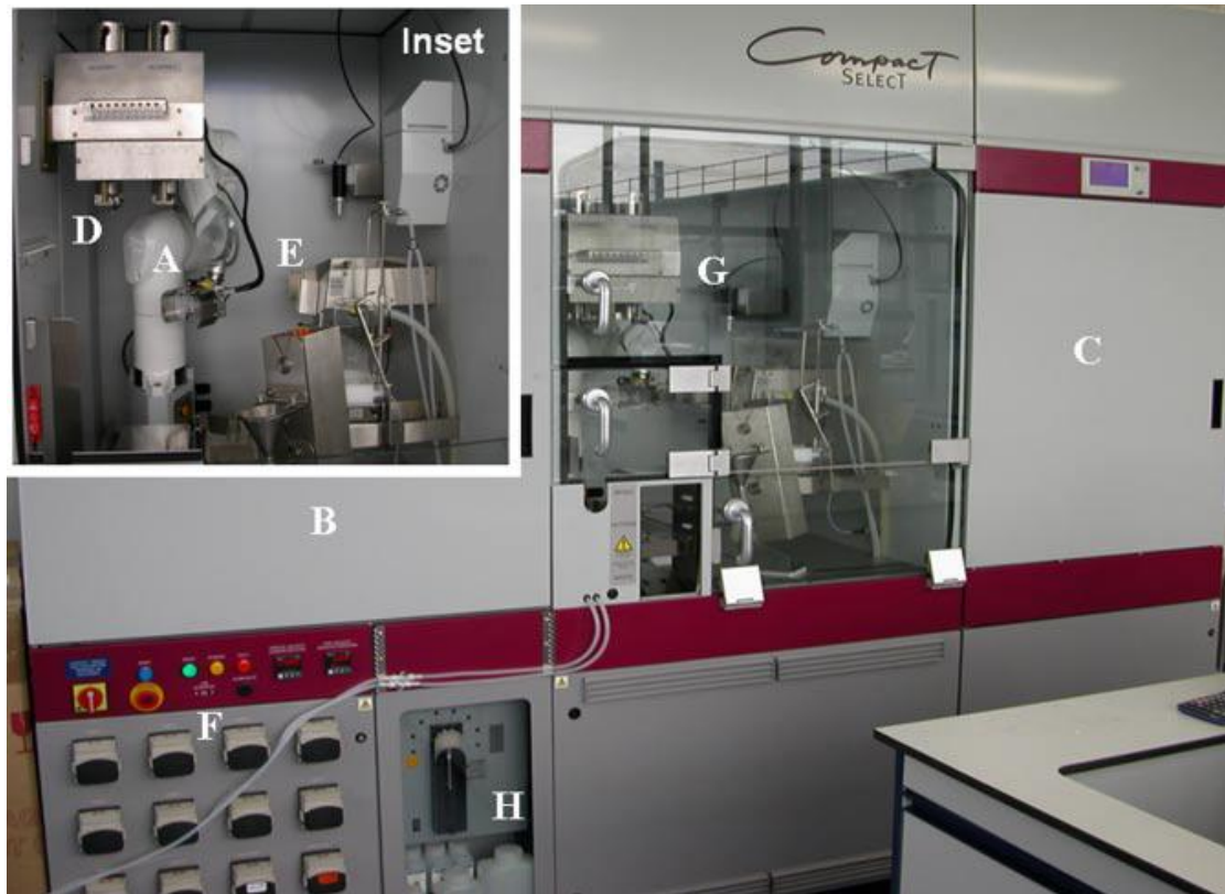
Figure 6-2: Features of the Compact Select. This automated cell culture platform can simultaneously manipulate 2xT175 flasks and house 90xT175 culture flasks in a robot-accessible incubator. All culture processes are carried out within a sterile class II environment and require no manual intervention. The inset shows an enlarged image of the manipulation chamber and pipette head. Major processing components are labelled: A, Robot arm; B, Flask incubator; C, Plate incubator; D, Flask decappers; E, Flask holders; F, Media pumps; G, Pipette head; H, Cedex automated cell counter
