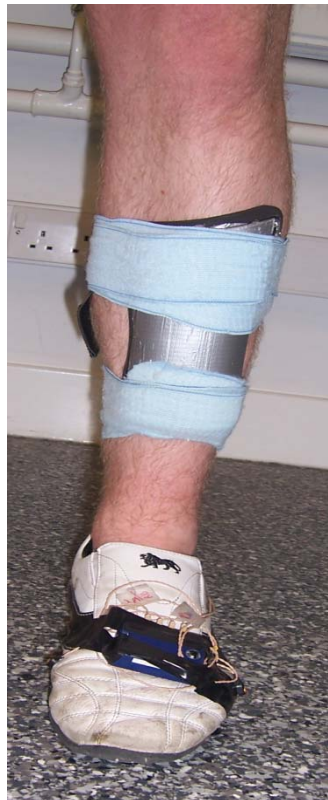
Figure 5.3: Positioning of the 0.9 kg mass for the WC tests
