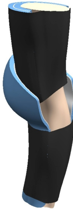
Figure 7. 6: Concept design including Nylon and Polyester straps.
