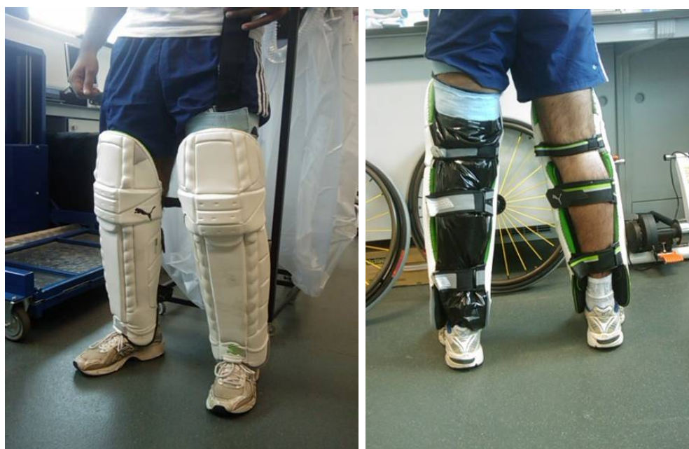
Figure 6. 4: Sensor mat mounted beneath pad on leading leg of cricketer
