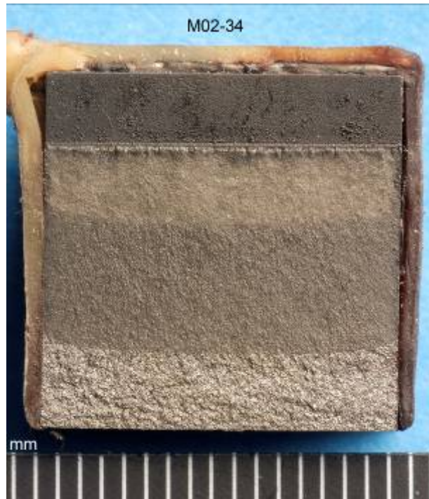
Figure 5.2 Discoloured fracture face from specimen coated such that only the back face was exposed to the sour environment.
