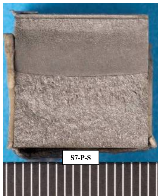
Figure 4.18 Fracture face from specimen S7-P-S tested under constant \Delta K conditions ( \sim 300 \text{ Nmm}^{-3/2} / \sim 9 \text{ MPam}^{0.5} ) after a one week pre-soak in the sour environment and with single-sided exposure (mm scale shown) (Holtam et al., 2010d).
