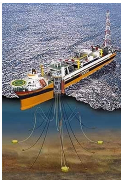
Figure 1.1 Floating Production, Storage and Offloading vessel, illustrating subsea pipelines and risers (image courtesy of Maritime Pusnes AS).
