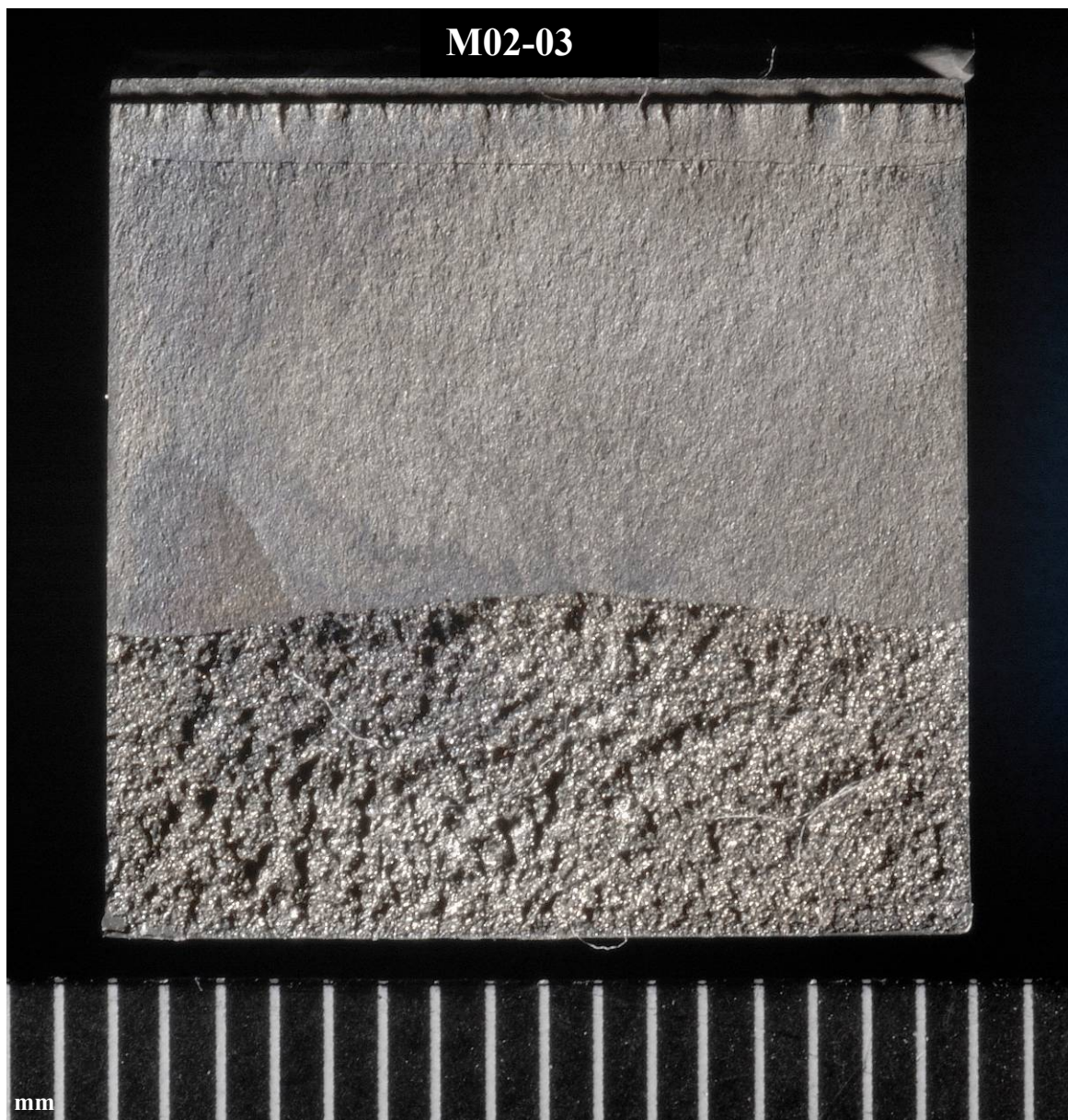
Fig. 7. Specimen M02-03 fracture face (decreasing \Delta K in a sour environment). Time spent in the sour environment: 31 h.
