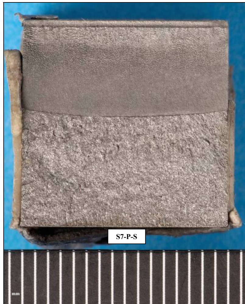
Fig. 11 Fracture face from specimen S7-P-S tested under constant \Delta K conditions ( \sim 300 \text{ Nmm}^{-3/2} ) after a one week pre-soak in the sour environment and with single-sided exposure.
