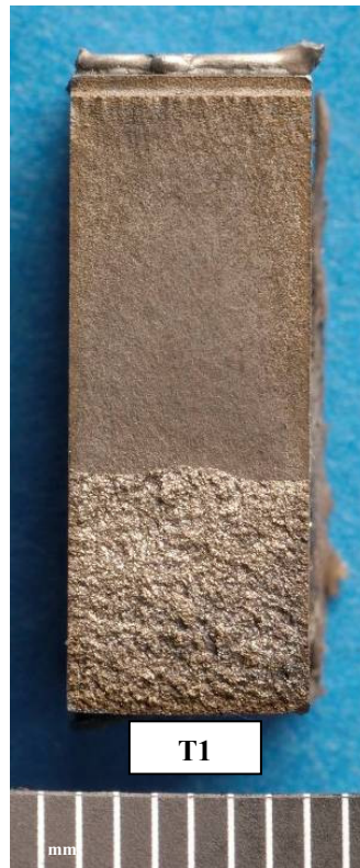
Fig. 8 Fracture face from thin specimen T1 tested under constant \Delta K conditions ( \sim 300 \text{ Nmm}^{-3/2} ).
