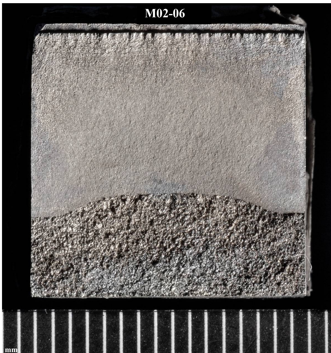
Fig. 9. Specimen M02-06 fracture face (constant \Delta K in a sour environment). Time spent in the sour environment: 216h.
