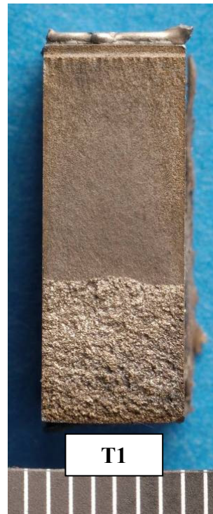
Figure 4.13 Fracture face from thin specimen T1 tested under constant \Delta K conditions ( \sim 300 \text{ Nmm}^{-3/2} / \sim 9 \text{ MPam}^{0.5} ) (mm scale shown) (Holtam et al., 2010d).
