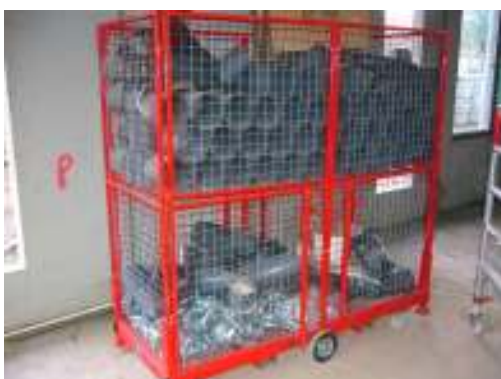
Figure 4.35 Mobile carrier for pipework components, type B materials (MTS)
