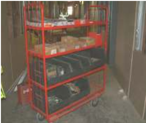
Figure 7 Mobile component trolley, with simple manual replenishment
