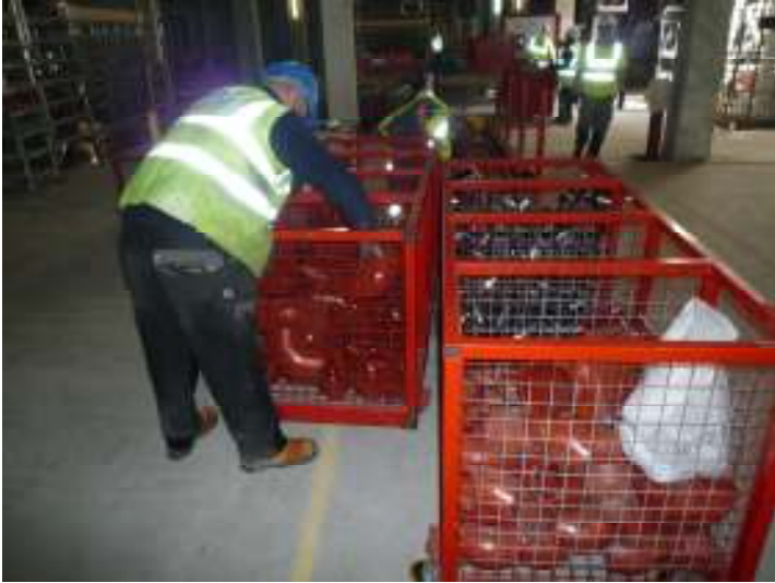
Figure 6.1 Mobile kanban unit for cast iron drainage fittings
