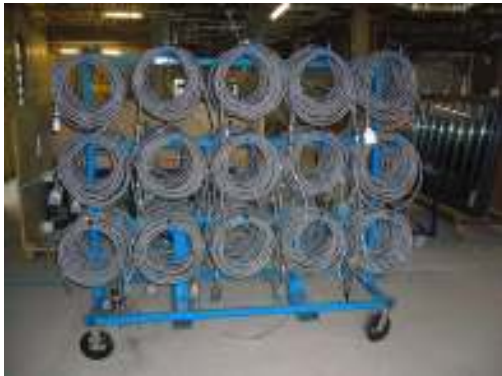
Figure 4.37 Mobile carrier for modular wiring components, type B materials (MTO)
