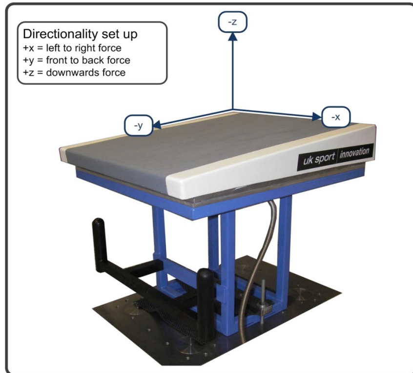
Figure 4-13: Orientation of axes on instrumented start block
