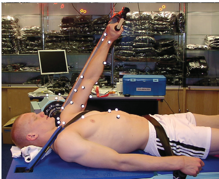
Figure 5.3. Dynamometer set-up to obtain shoulder torque measurements.
