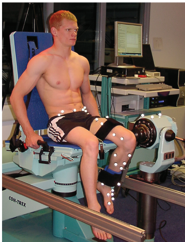
Figure 5.1. Dynamometer set-up to obtain knee torque measurements.
