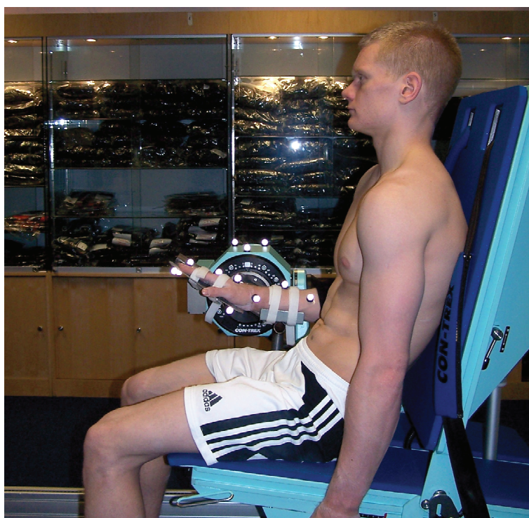
Figure 5.4. Dynamometer set-up to obtain wrist torque measurements.
