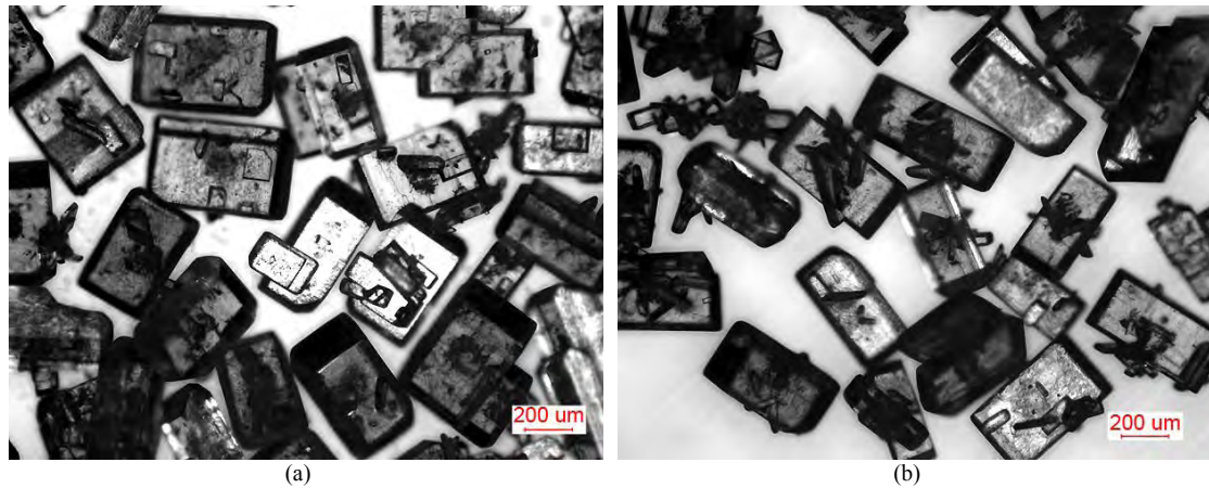
Figure 8.18: Microscopic images for the products at the end of the batches a) experiment C (180 minutes) and b) experiment D (90 minutes).
