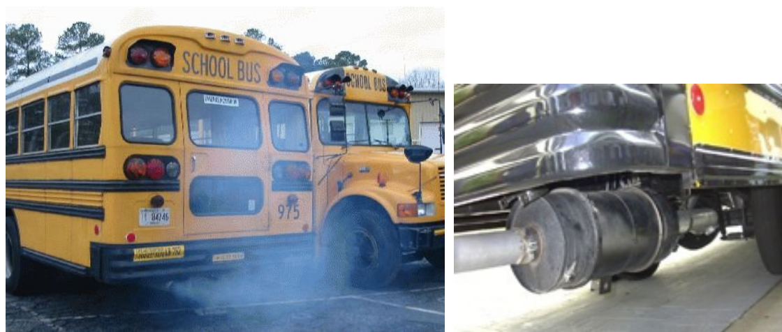
Figure 1.2 The known dangers of particulate inhalation has led to the retrofiting of DPF technology ( right ) on vehicles such as school buses
