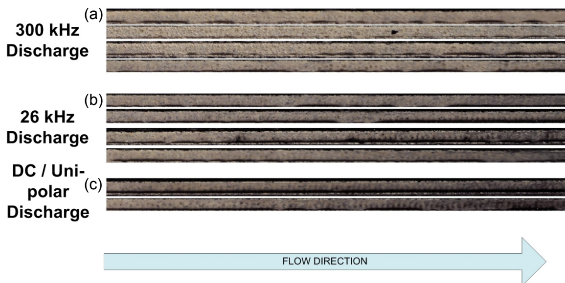
Figure 5.8 Scan of filter sections showing channel blackening on the clean (downstream) part of the filter. Blackening increases gradually towards the downstream end of the channels. (a) is the result of a 300 kHz discharge, (b) results from 26 kHz and (c) from a DC discharge
