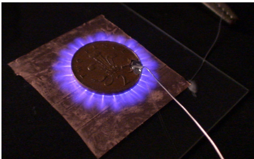
Figure 3.7 A dielectric barrier discharge, the dielectric is a glass sheet between the coin and copper foil ground plane
