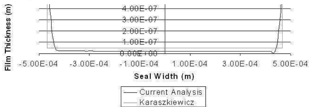
Figure 7.3: Typical contact film thickness/seal profile
