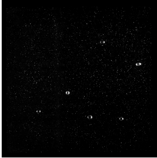
Figure 5.4: Background-subtracted PIV image
