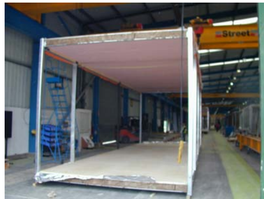
Figure 5.13 Modular building manufacture; floor cassette and wall elements
