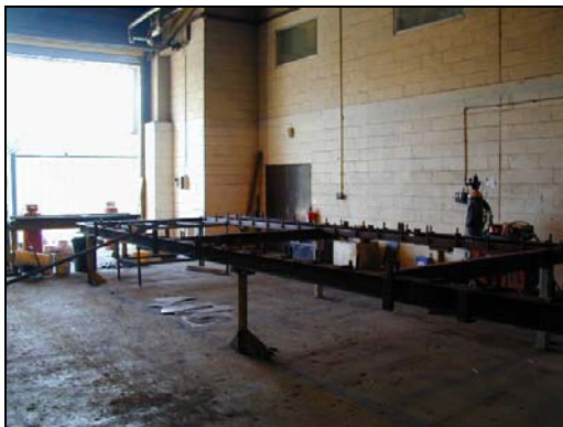
Figure 5.13 Modular building manufacture; floor cassette and wall elements
