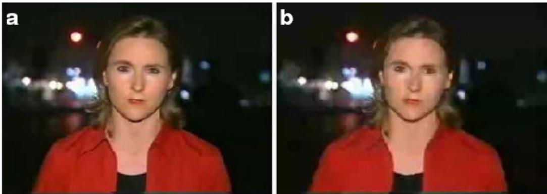
Figure 4-1: Sample image frame compressed with different compression parameters. (a) QP=30, I-Frame=2, B-Frame=2; (b) QP=40, I-Frame=2, B-Frame=2
