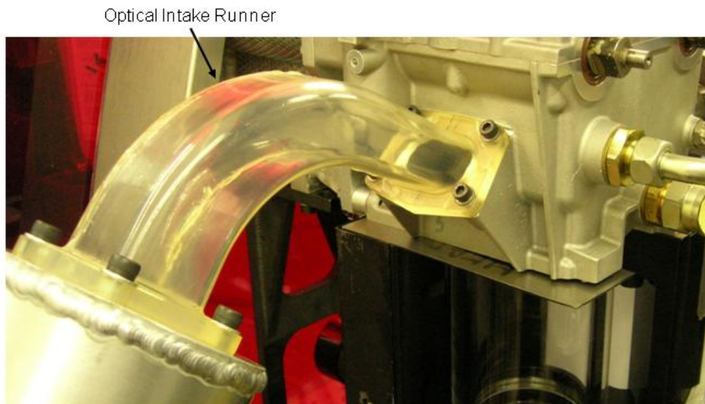
Figure 4.6 - Schematic of the optical intake
