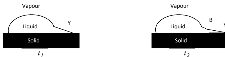
Figure 3.3 – Schematic diagram showing the change of curvature of the liquid droplet over time with t_1 < t_2 .
