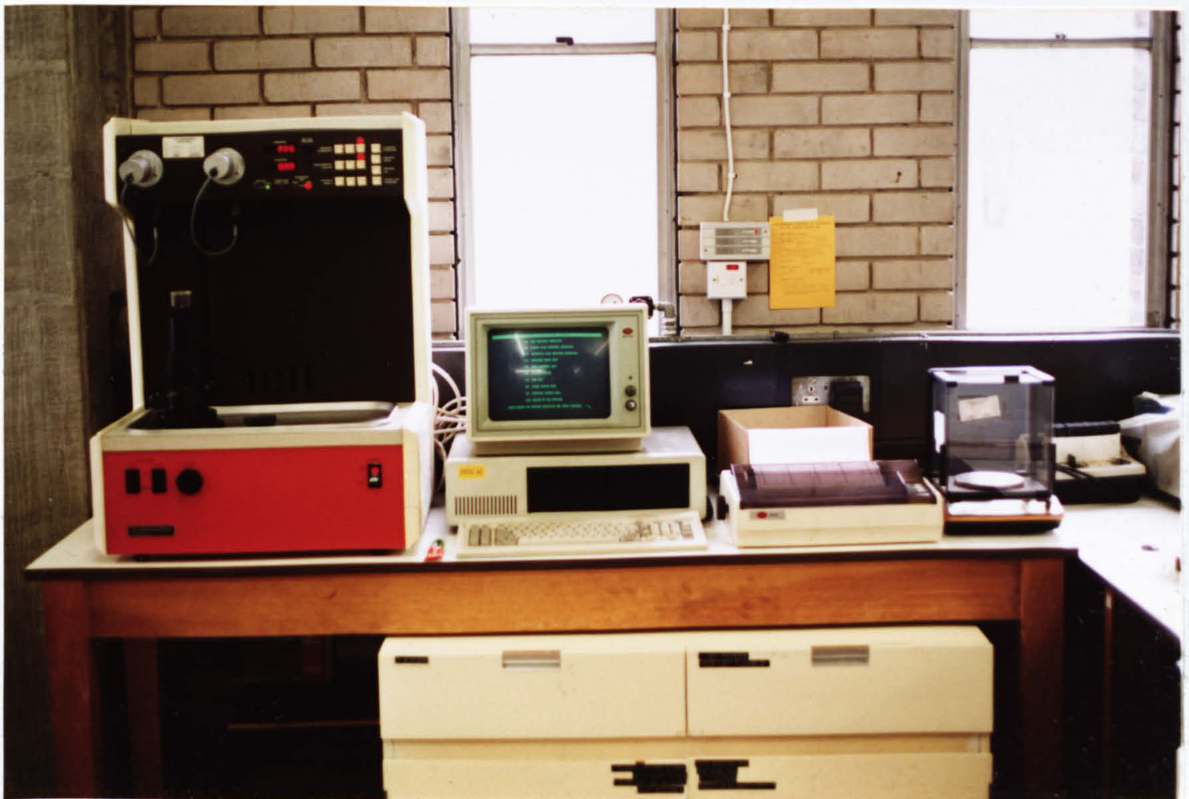
Plate 6.6 Pore size distribution test apparatus
