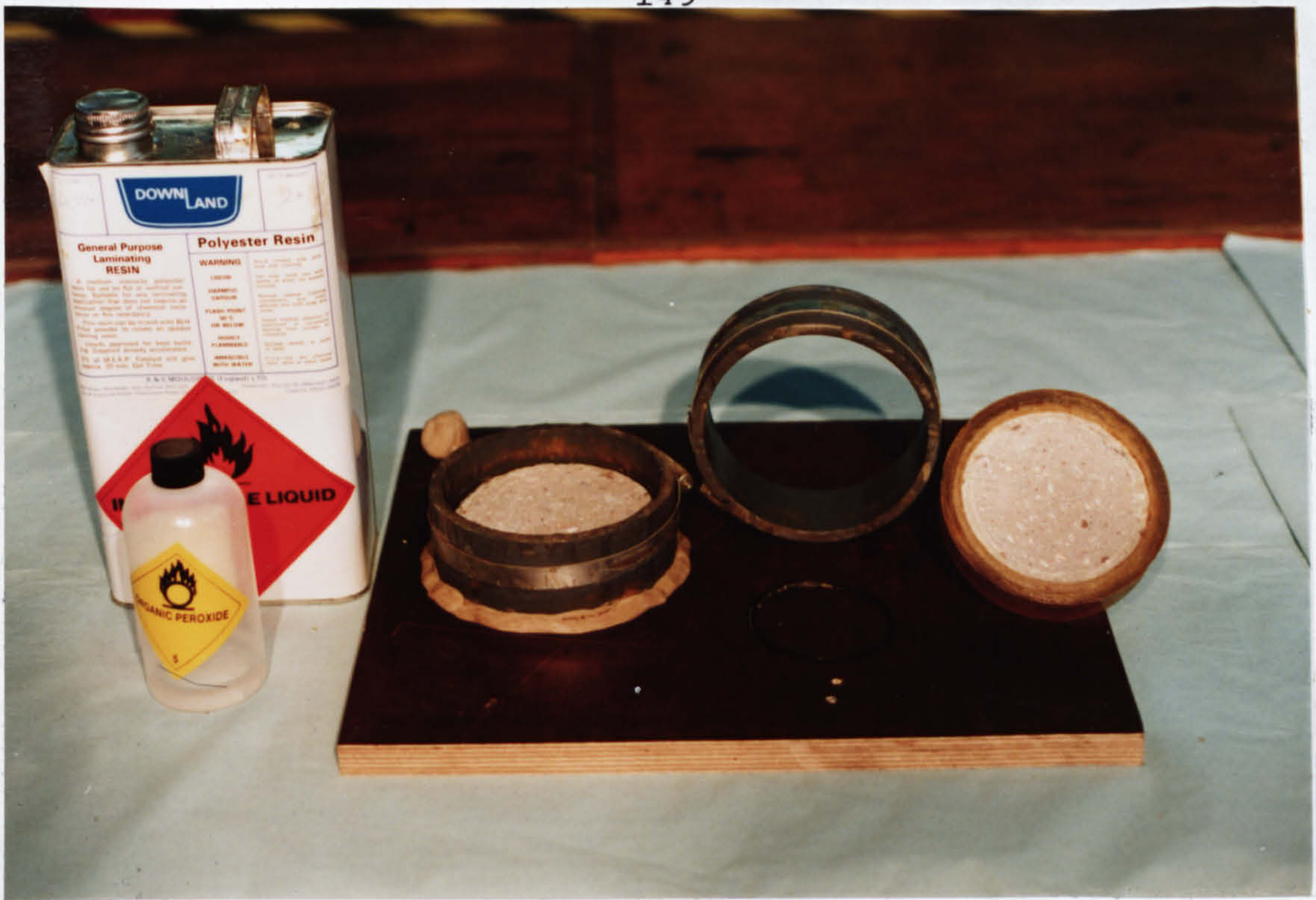
Plate 6.9 Preparation of test specimen for water permeability
