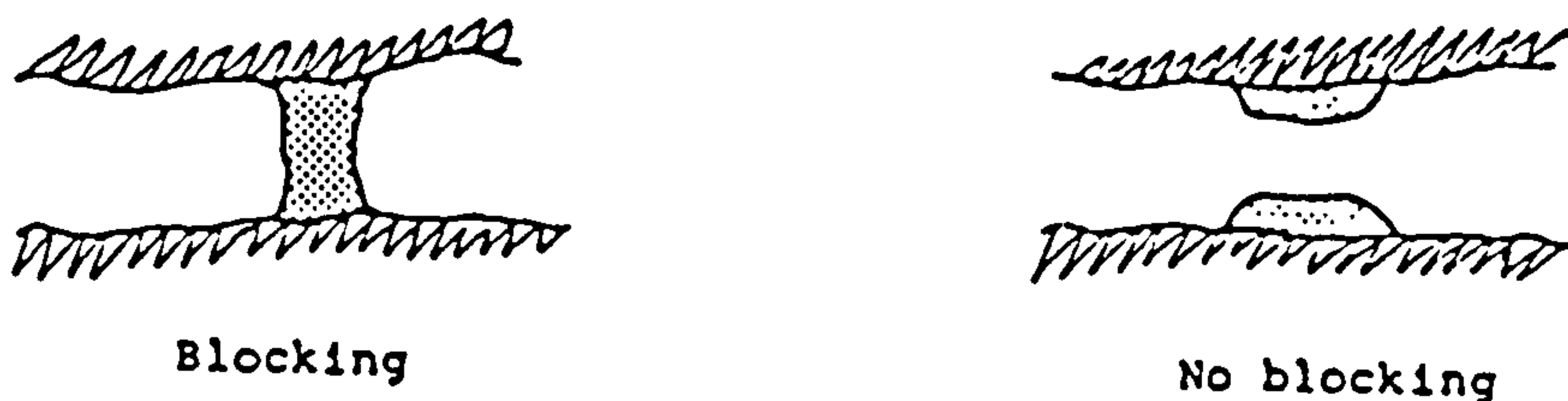
Figure 3.19 Influence of locality of precipitation of the same amount of gel on the sealing effects in a pore (102)
