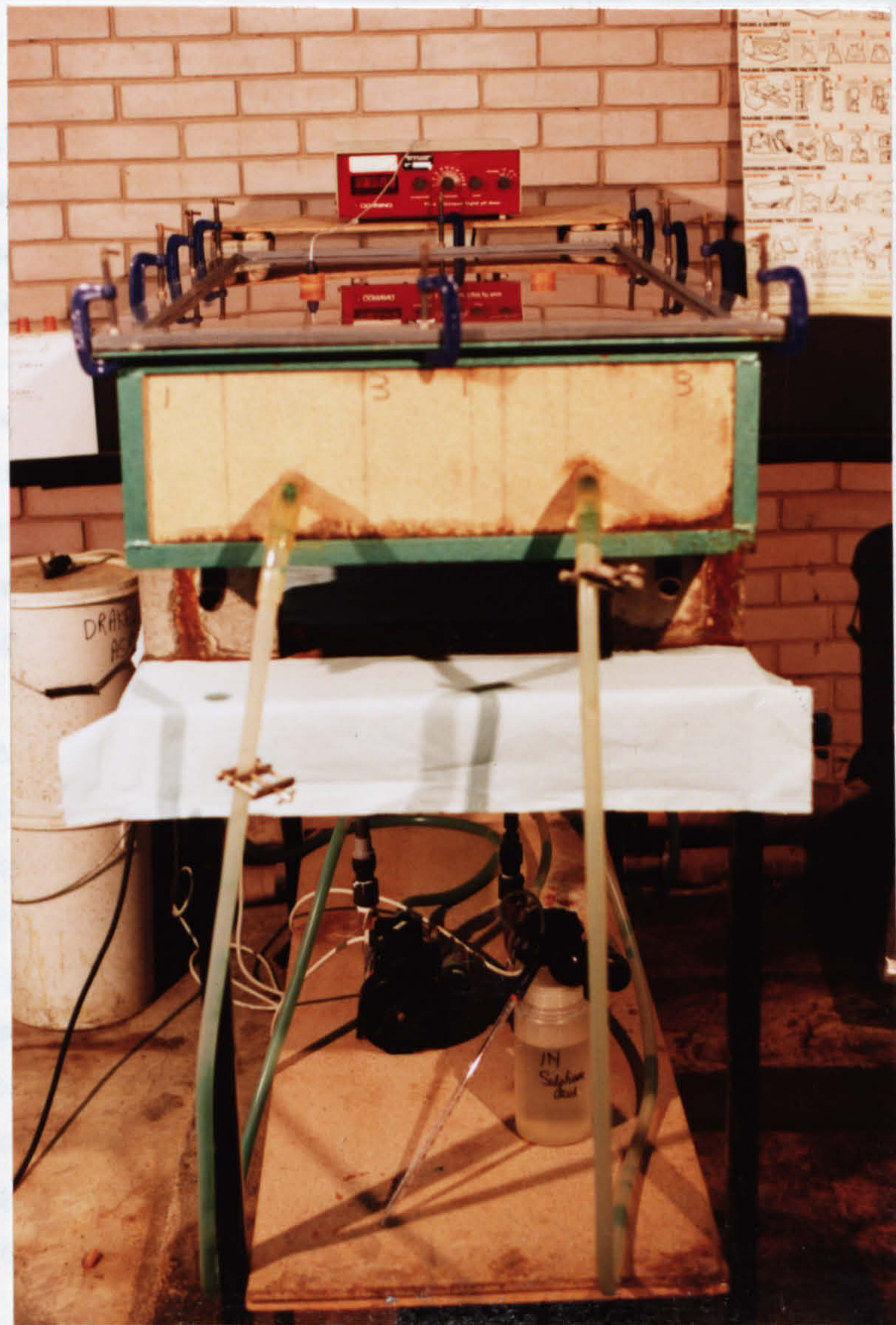
Plate 6.10 Apparatus used in the controlled environment sulphate attack test
