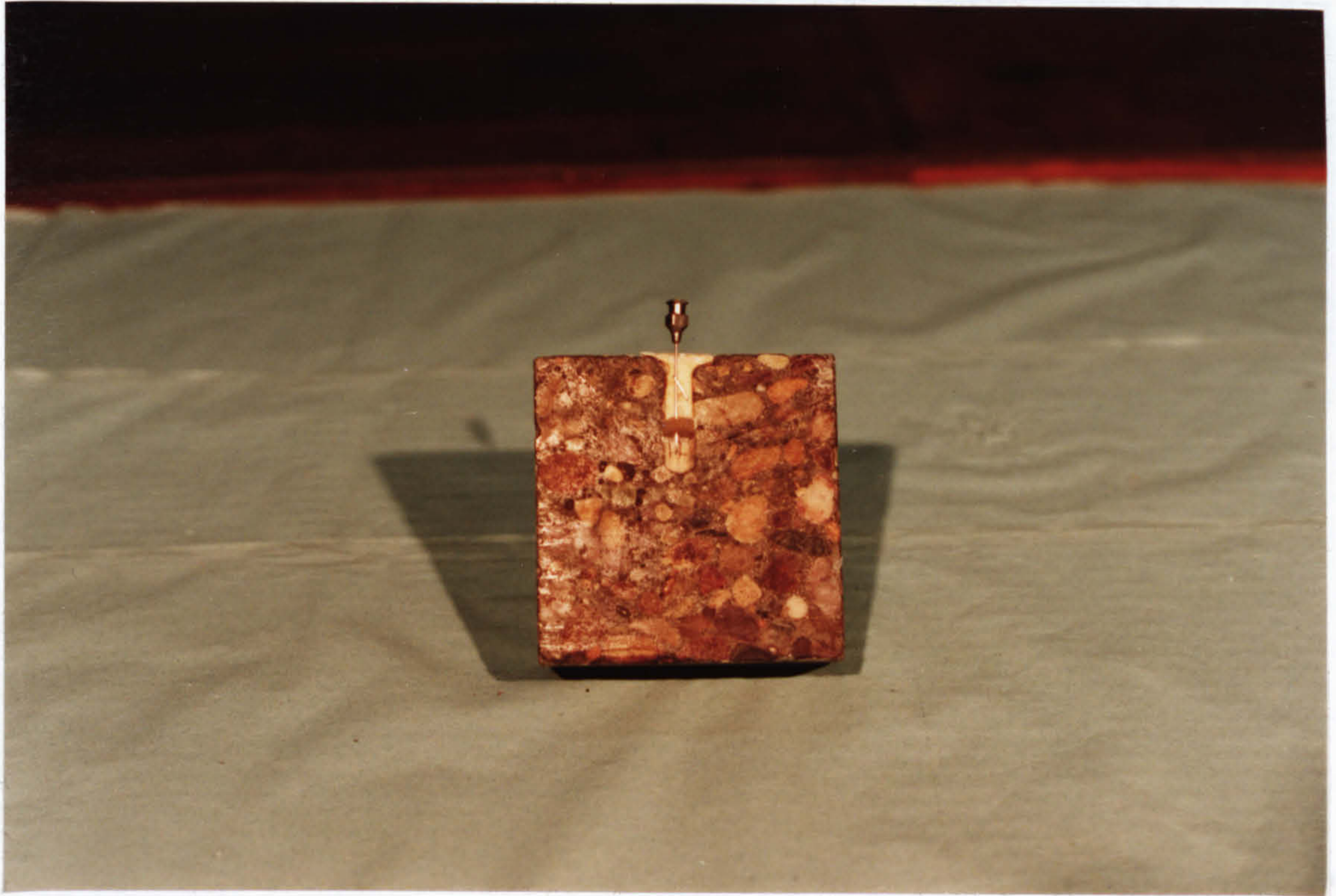
Plate 6.1 Figg test hole details
