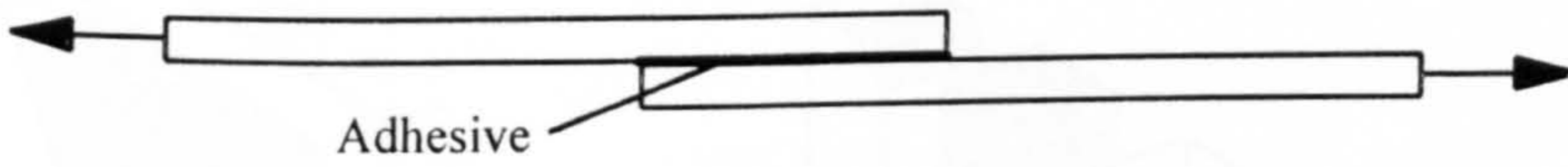
a) Single lap test
