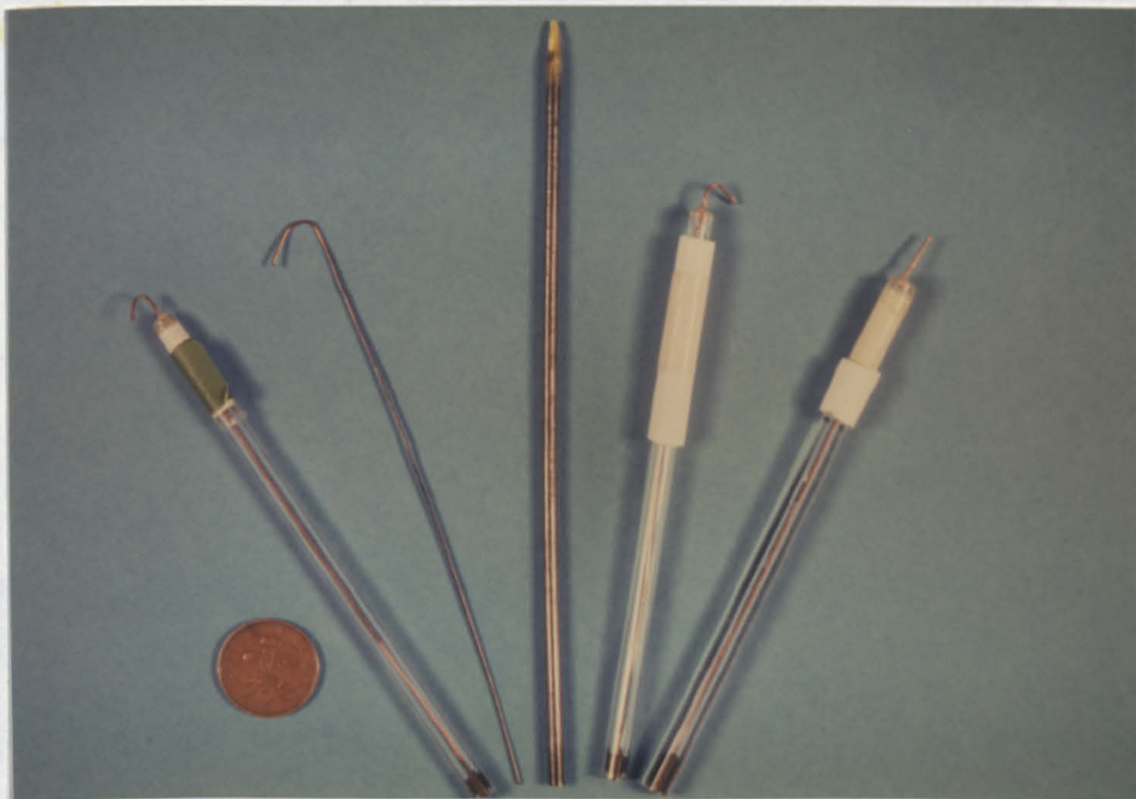
Fig. 32 Disc Electrodes Used in ASV Shown Together with a Coated Wire and a Coated Plastic Rod.
