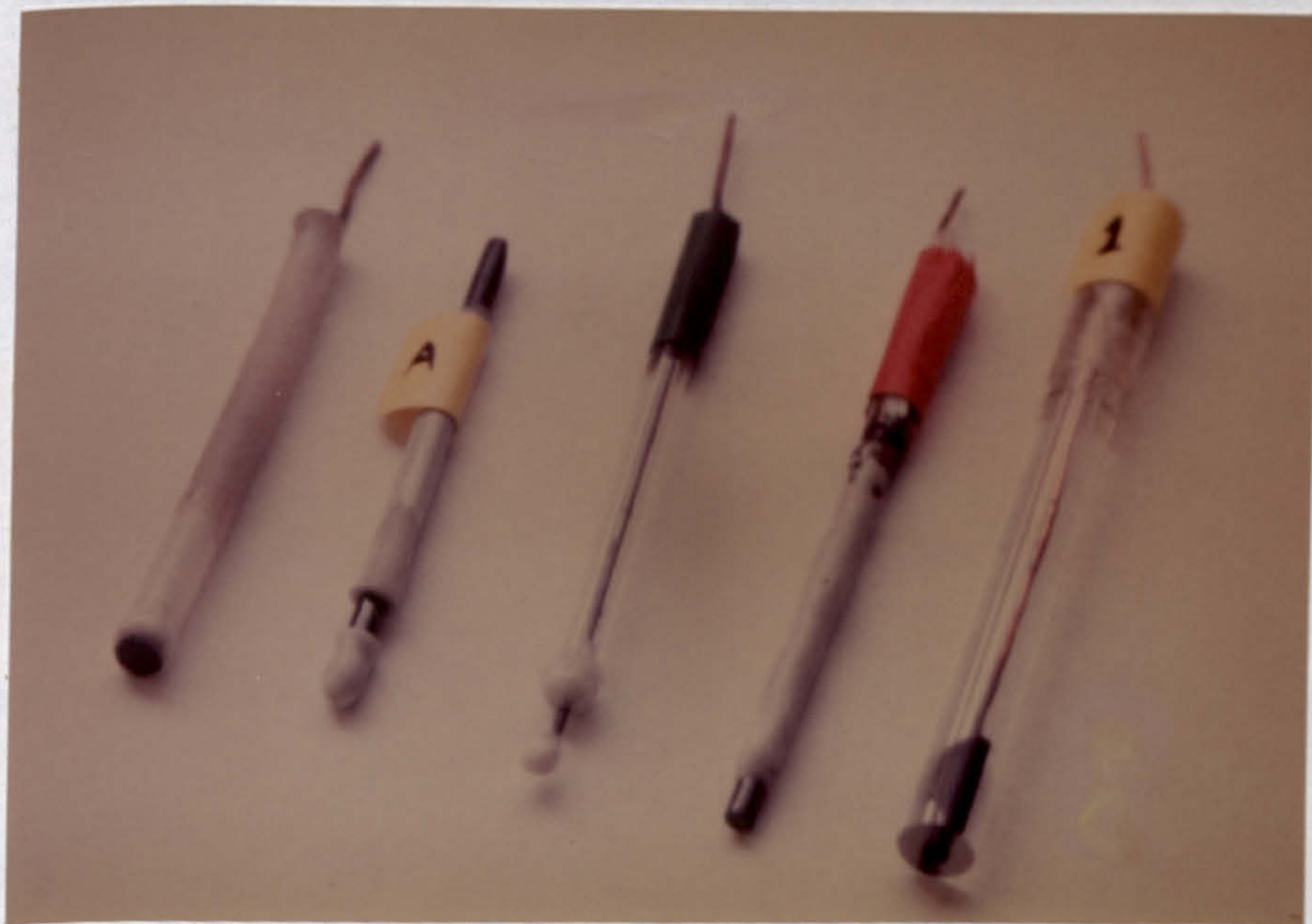
Fig. 30 Different types of Epoxy-based Voltammetric Electrodes.
