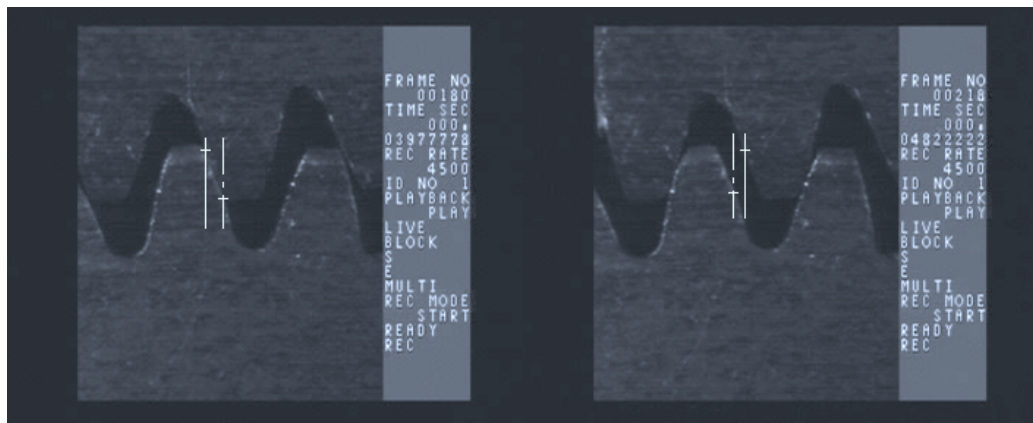
Figure 2.10 - Backlash measurement on consecutive tooth face impacts.
