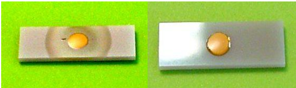
Figure 1-3 Epoxy bleed from thermally conductive boron nitride loaded epoxy, pronounced (left) and acceptable (right).
