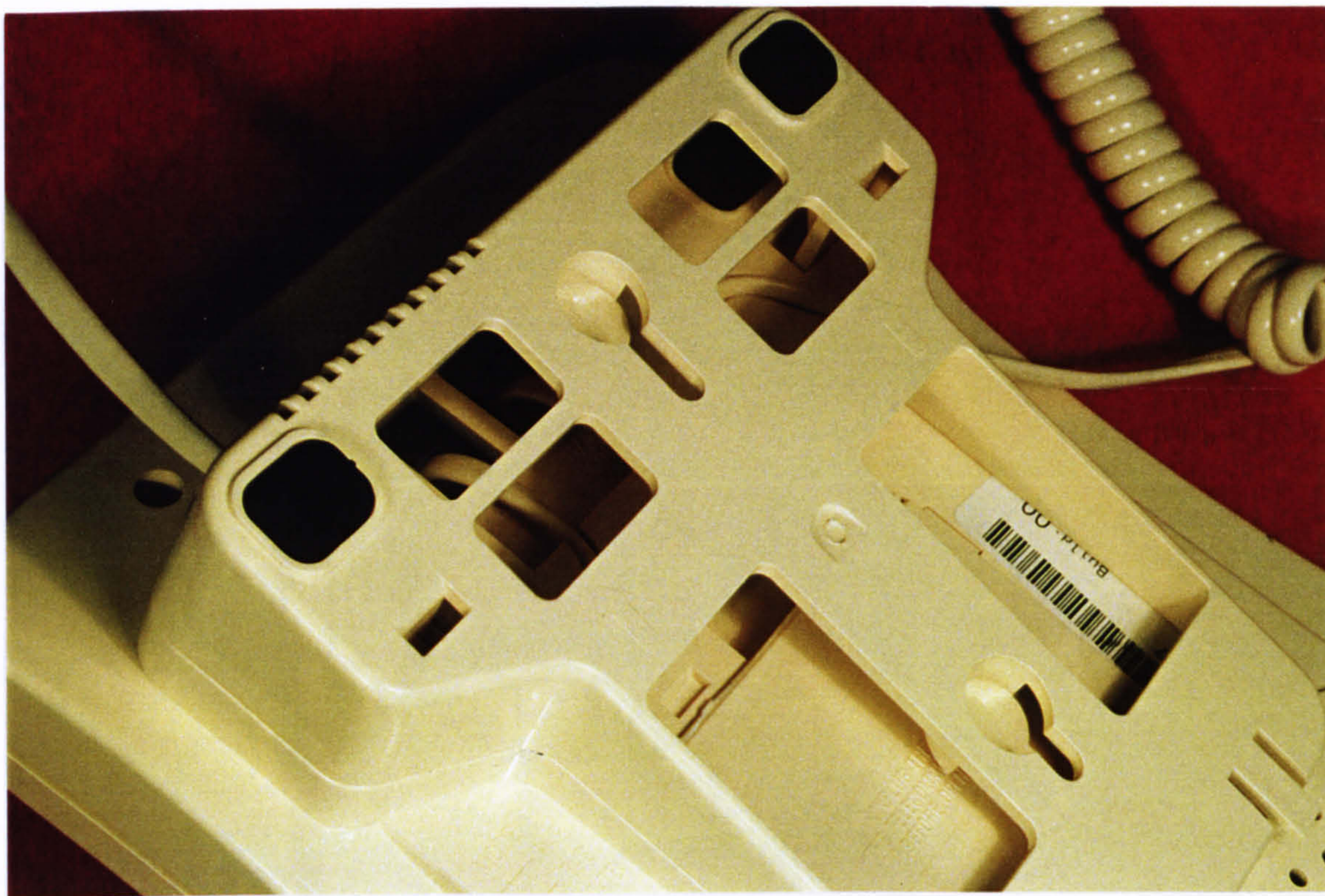
Figure 3.2 Presence of base stand restricting access to the removal of the line and handset cords
