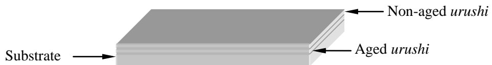
Figure 6.17: Schematic of the substrate and two urushi layers. The bottom layer is aged urushi layer, while the upper layer is non-aged urushi layer.
