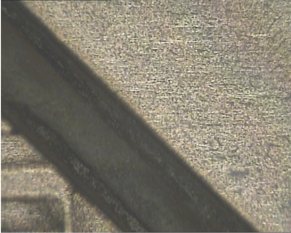
Figure 8-8: An image of a 45-degree 2D in-plane mirror filled with copper using electroplating.
