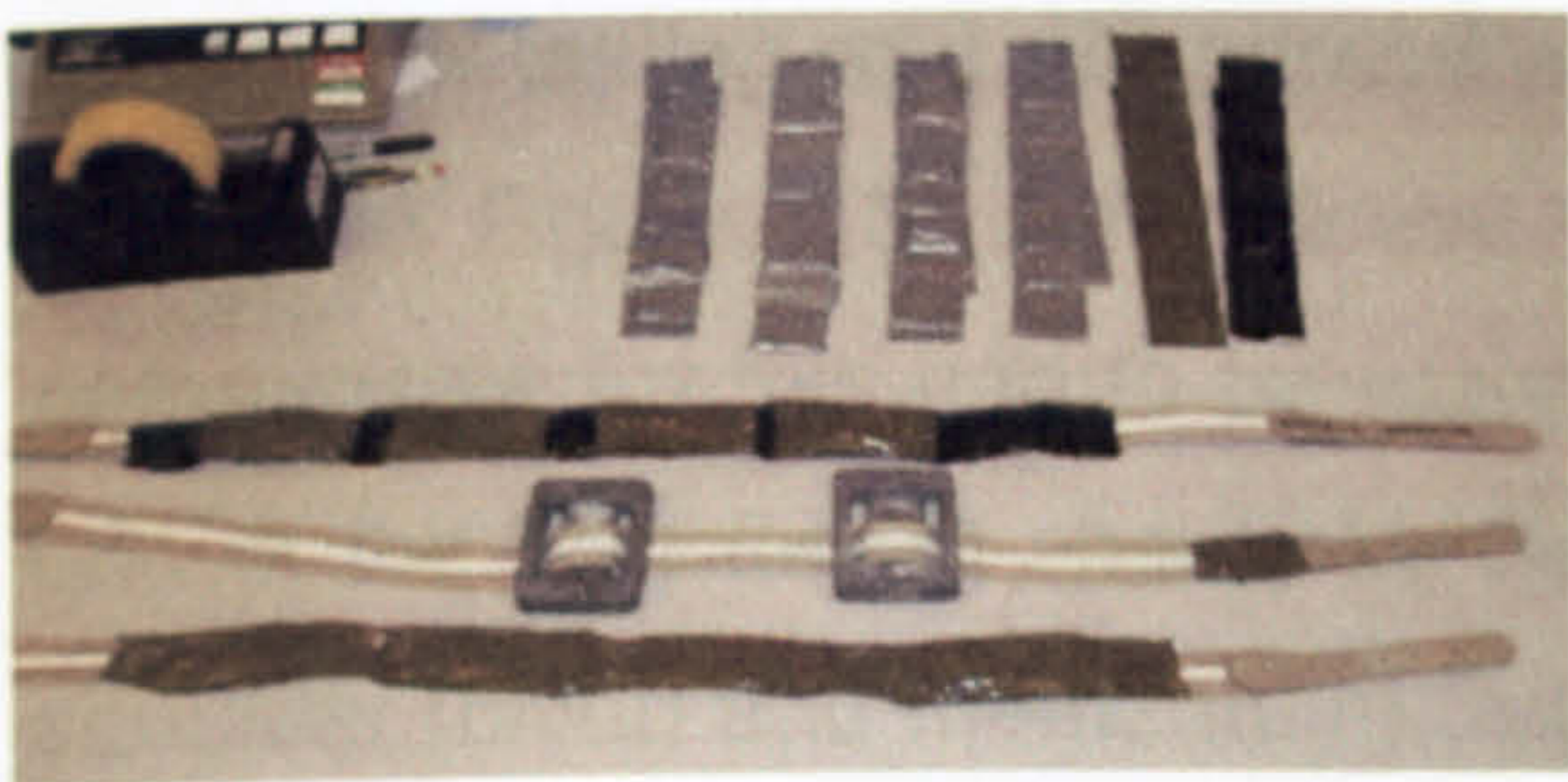
1. weights made up for the ankles and wrists using lead weight and tape (top of the photo) and belts for the waist with weights taped on (bottom of the photo).
