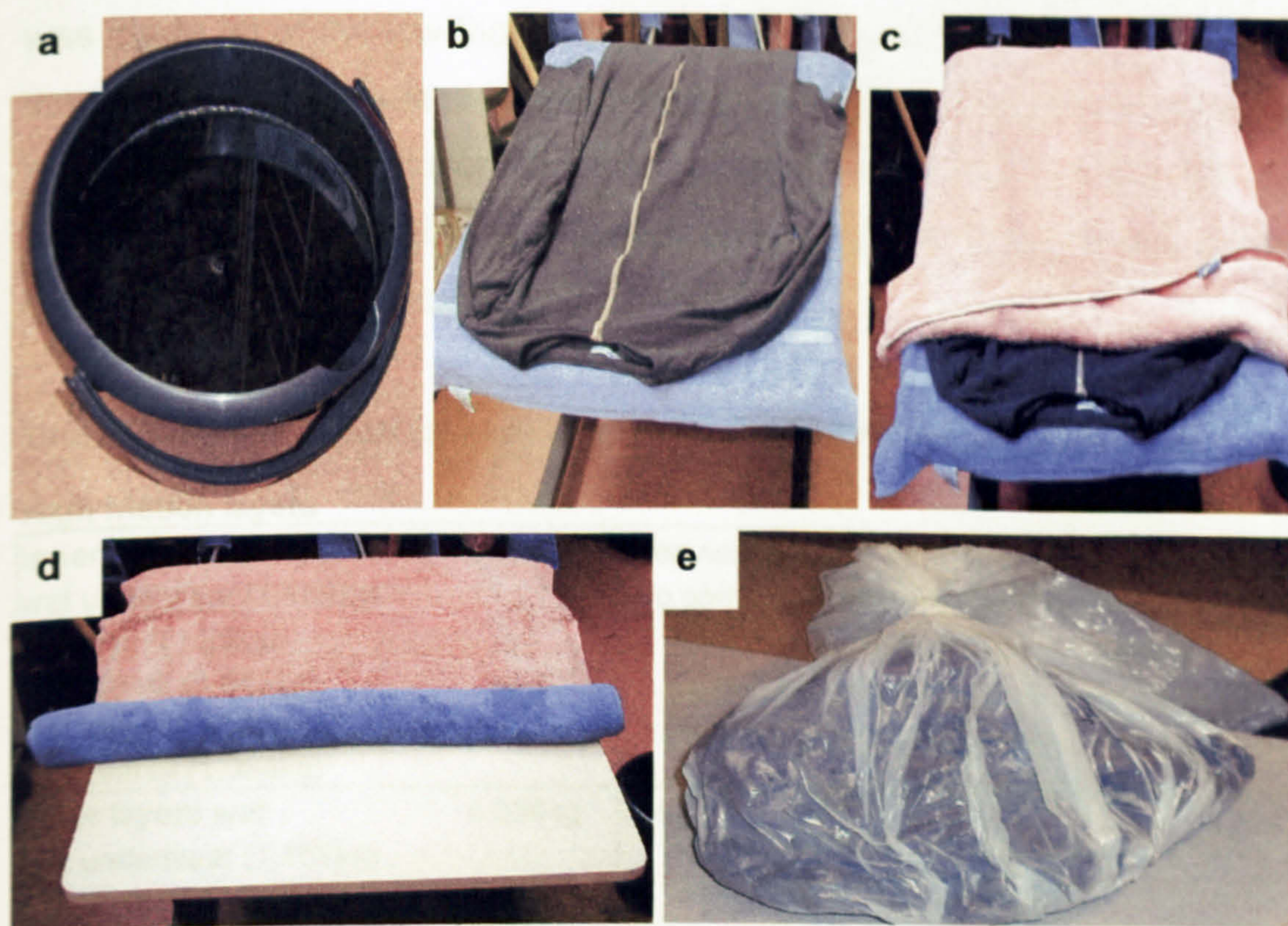
Figure 2.1. Process of wetting garments a. soaking of garment by immersing in bucket of water, b. laying of garment on towel, c. covering garment with second towel, d. rolling of excess water from garment and e. storage of wet garment in plastic bag.
