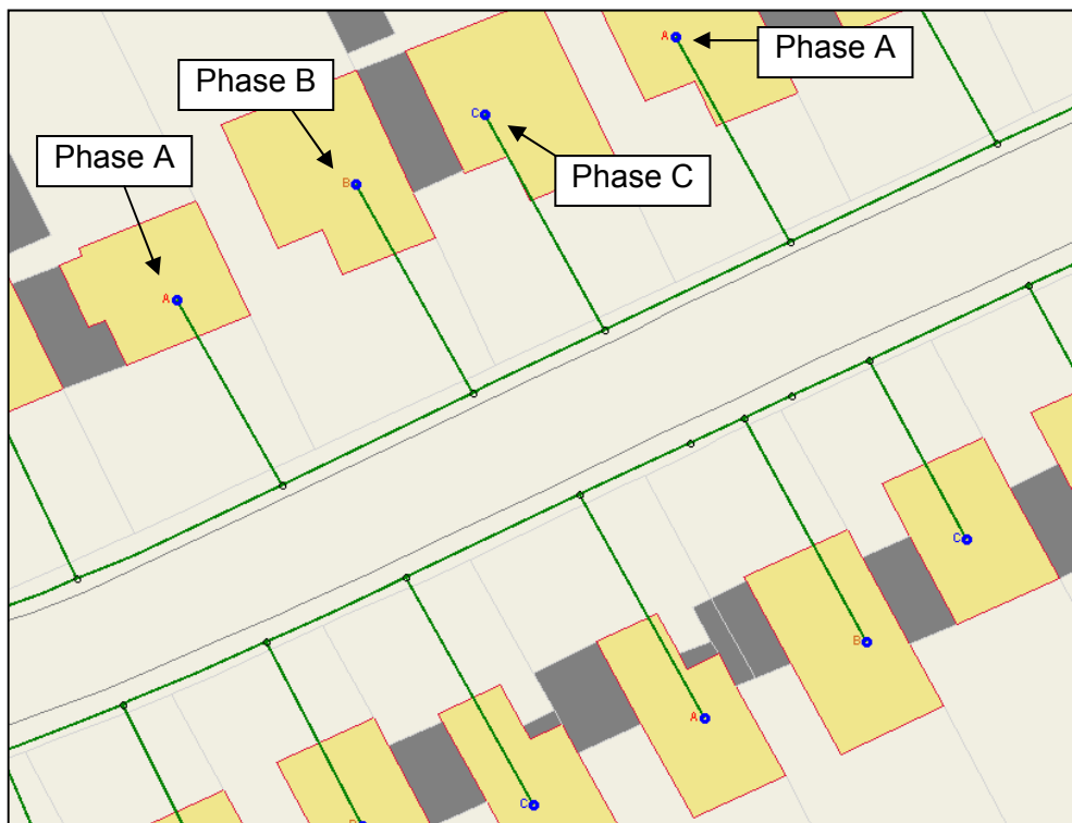
Fig. 65. Assignment of connection phases
