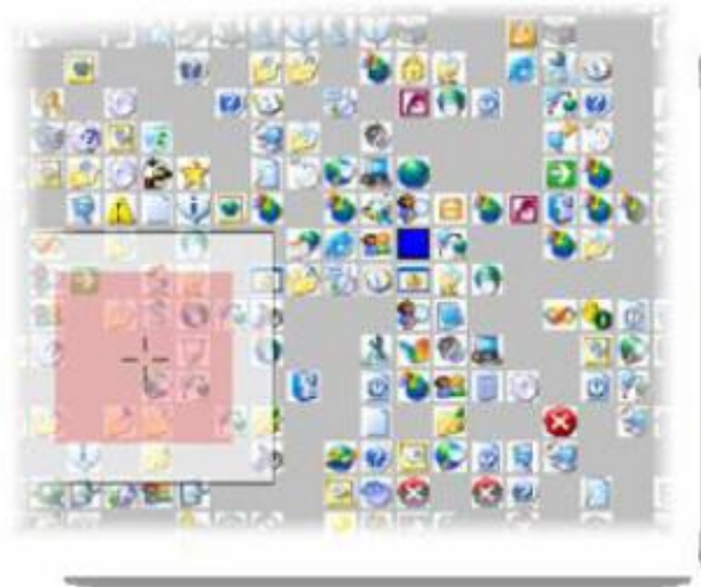
Figure 26: Two-step magnification technique. The square represents the area which will be magnified by using dwell. (Skovsgaard et al., 2008).
