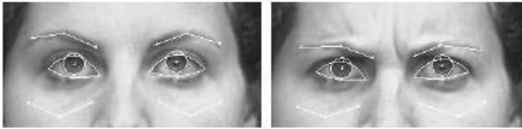
Figure 9: Feature point tracking using the iris and shape of eyes (Tian et al., 2000)
