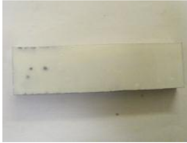
Figure 6.9. The sample used for the rough surface measurement test consisting of an aluminium block spray painted with white metallic paint
