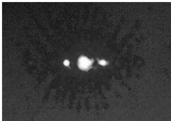
Fig. 4-27: Image of the focal spot magnified 100x over a distance of approx .2m
