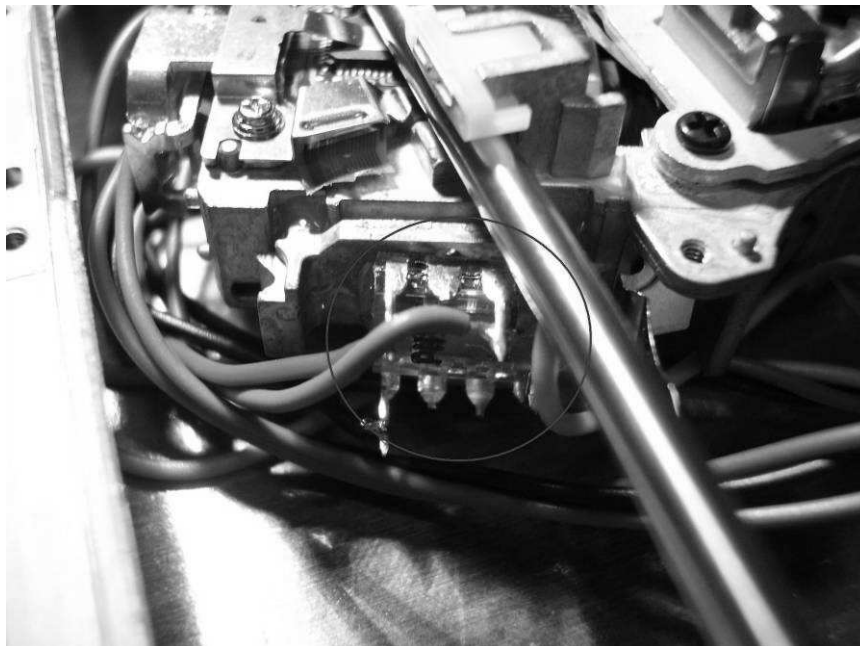
Fig. 4-50: OPT 101 mounted in optical pickup unit (red circle)
