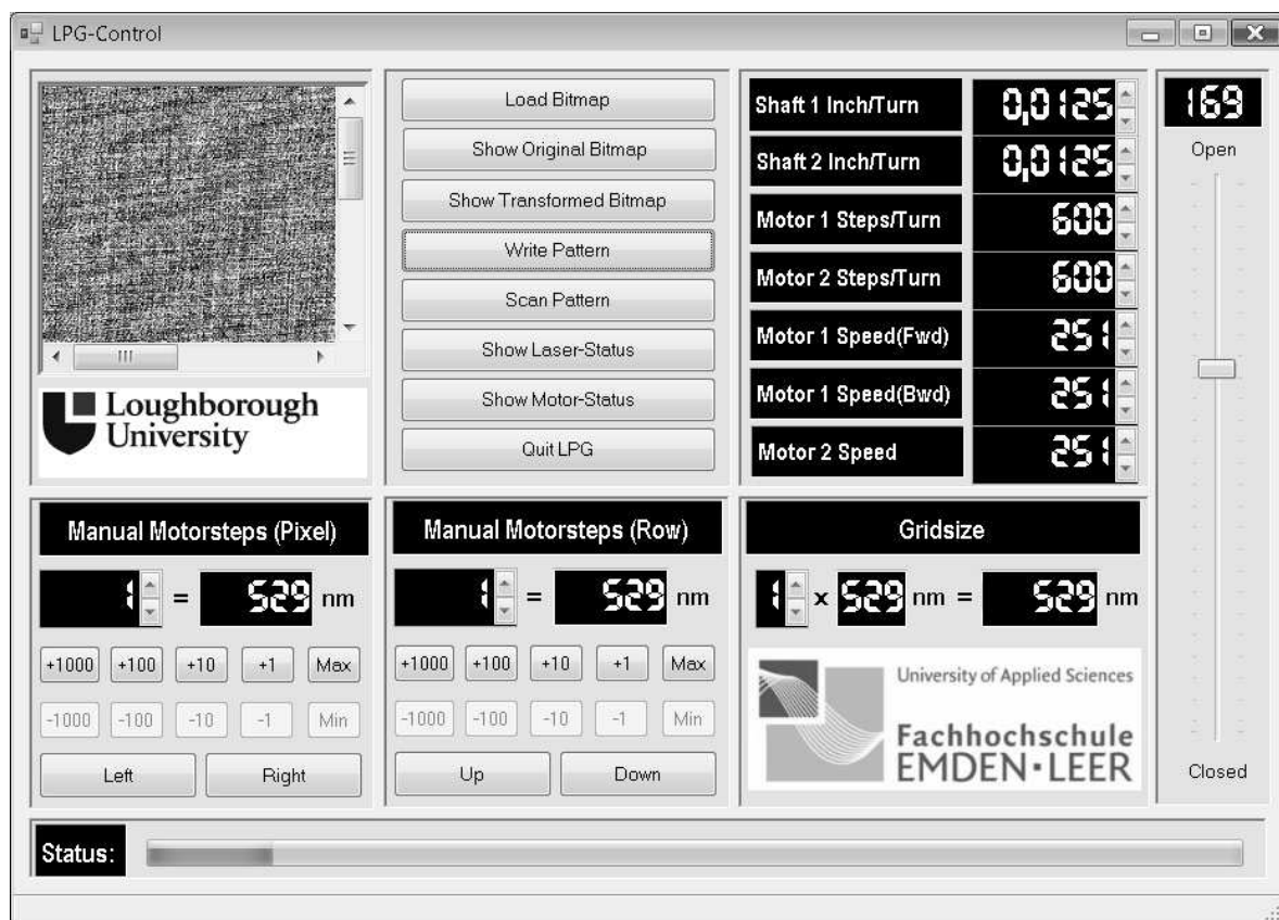
Fig. 6-21: Screenshot of the main screen of the controlling software
