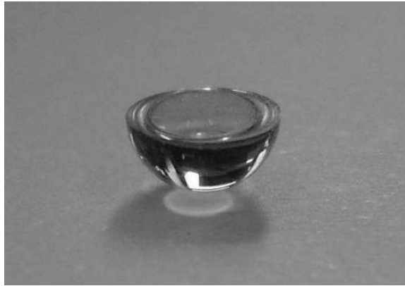
Fig. 5-1: Example of hemispherical SIL made of BK7- glass (diameter 2mm; height 1mm)
