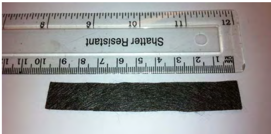
Fig. 19. Carbon fibre mat comprising short carbon fibres (SF), which are randomly orientated.
