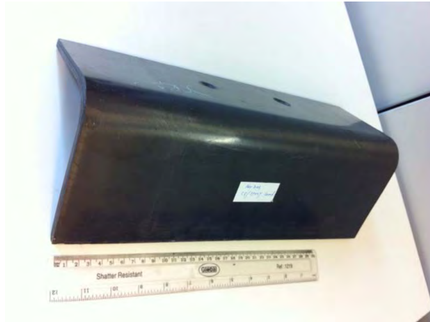
Fig. 20. Photograph of the cured CFRP spar.
