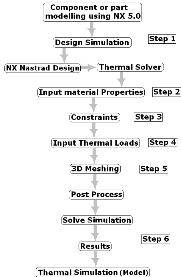
Figure 7.1 A schematic diagram of the steps taken to construct the FEM.
