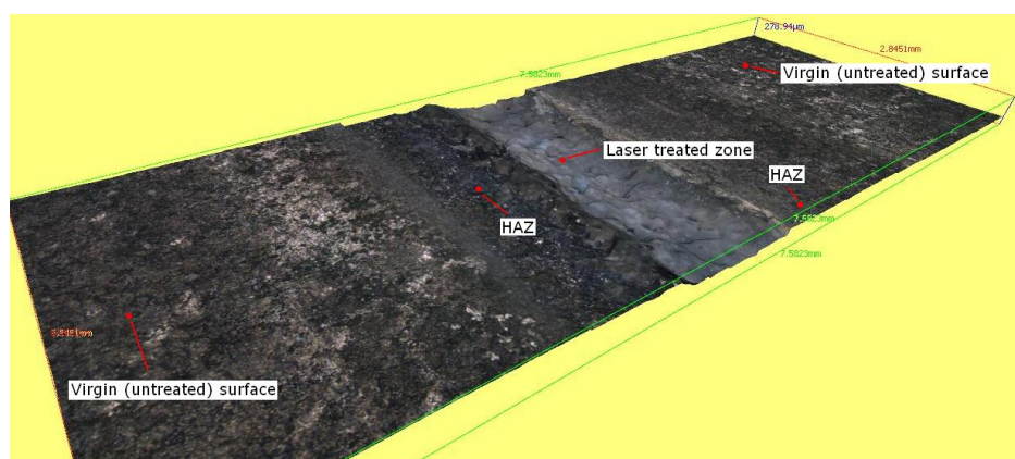
Figure 5.4 A 3-D topographical image of the surface profile of the Si 3 N 4 engineering ceramic treated by the fibre laser irradiation by using an O 2 assist gas.
