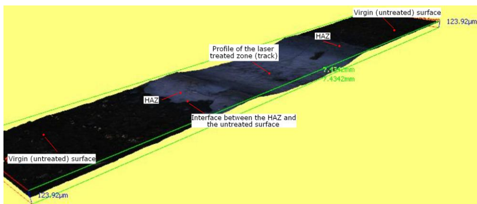
Figure 5.25 A 3-D topographical image of the surface profile of the \text{Si}_3\text{N}_4 engineering ceramic treated by \text{CO}_2 laser irradiation by using compressed air assist gas.
