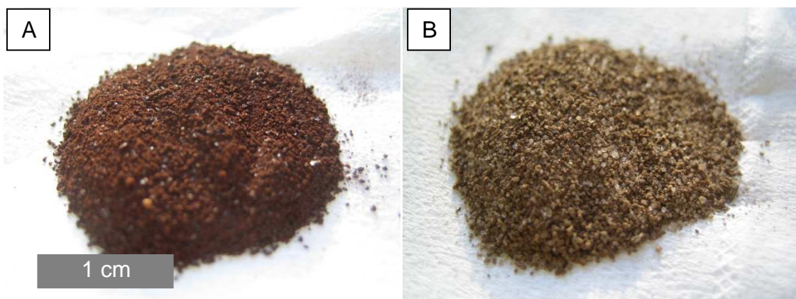
Figure 3. Ashes from ST (A) and CE (B) sludges (17 h at 400 °C).
