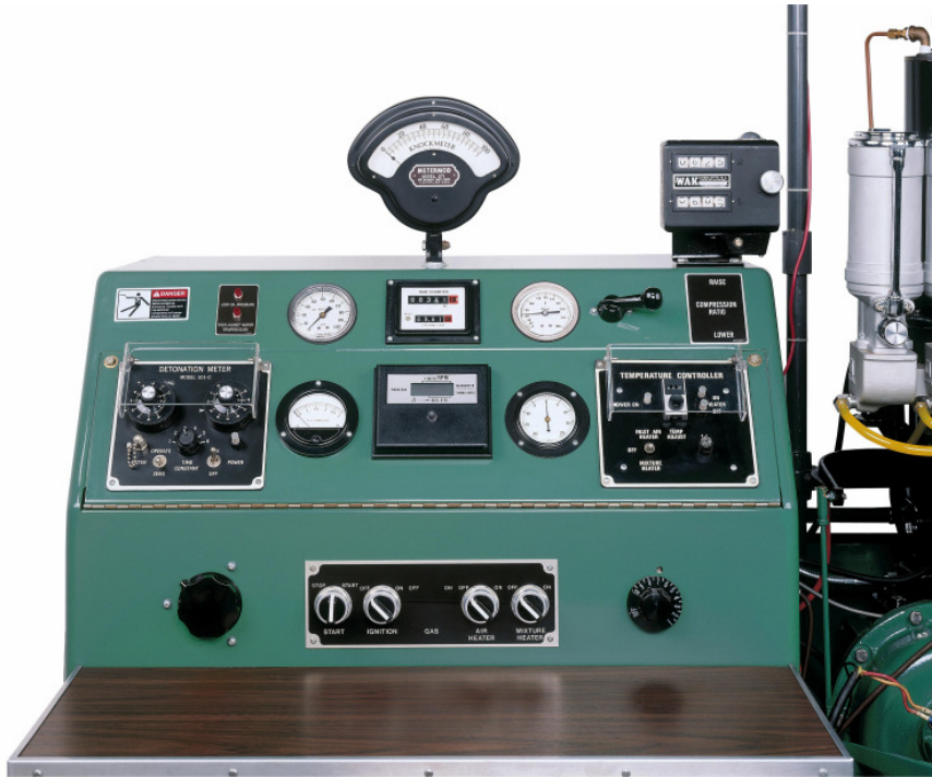
Fig. A3.3: Analogue control panel for the CFR™ fuels rating engine in F1/F2 specification for RON and MON testing. The knockmeter readout is positioned at the top. This control panel has just been superseded by the XCP Digital Octane Panel (Website, 2011b). (Photograph provided compliments of DresserWaukesha)
