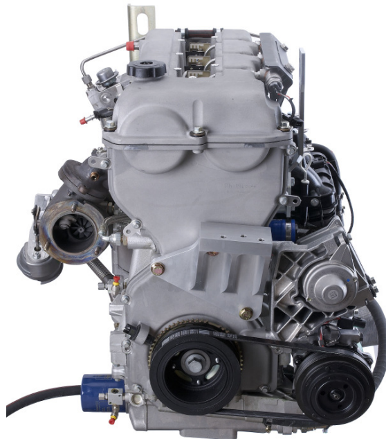
Fig. 7.5(b): Photograph of left hand (intake) side of Sabre 3-cylinder downsized demonstrator engine. (Photograph courtesy Lotus Engineering)
