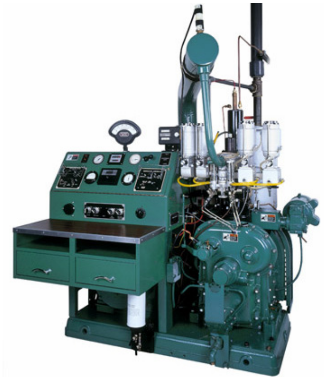
Fig. 3.4: The CFR™ variable compression ratio test engine, adopted as the standard fuels rating engine across the automotive and petroleum industries.
