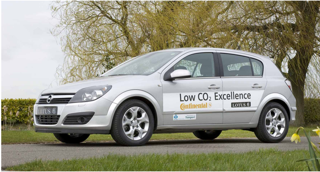
Fig. 7.7: GM Astra test vehicle fitted with Sabre downsized demonstrator engine. (Photograph courtesy Lotus Engineering)
