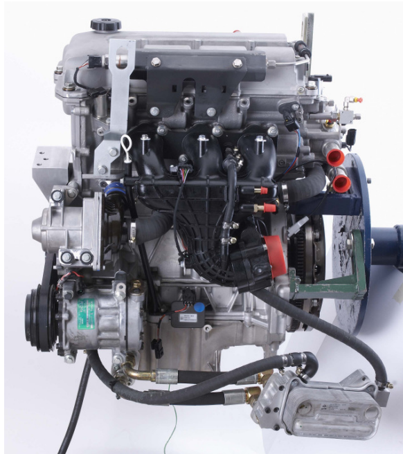
Fig. 7.5(b): Photograph of left hand (intake) side of Sabre 3-cylinder downsized demonstrator engine. (Photograph courtesy Lotus Engineering)
