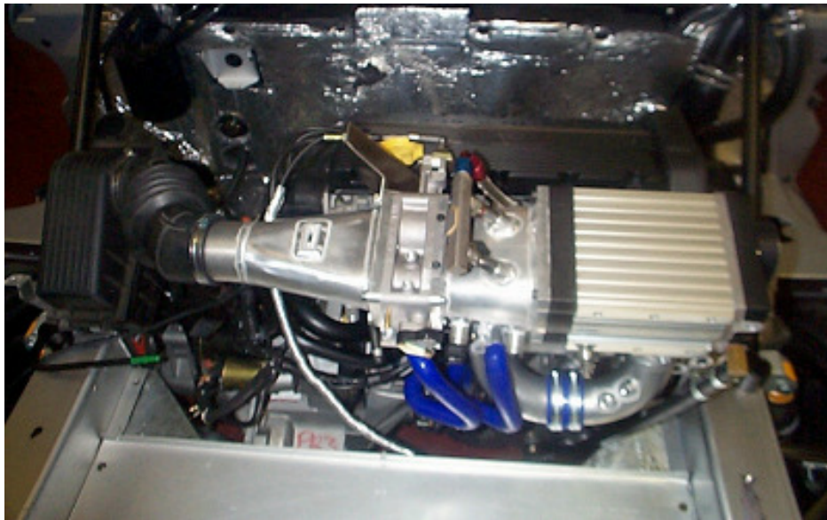
Fig. 2.5: Development engine application of Opcon AB twin-screw compressor on Rover K-Series engine, employing pre-compressor injection in place of charge air cooling and described by Turner and Pearson (2001). The pre-compressor injectors are visible and positioned at the entry to the supercharger rotors. (Photograph courtesy Lotus Engineering)
