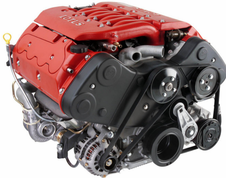
Fig. 2.9: Photograph of a Lotus Type 918 V8 engine. The turbocharger for the right-hand cylinder bank is visible beneath the right-hand cylinder head. (Photograph courtesy Lotus Engineering)
