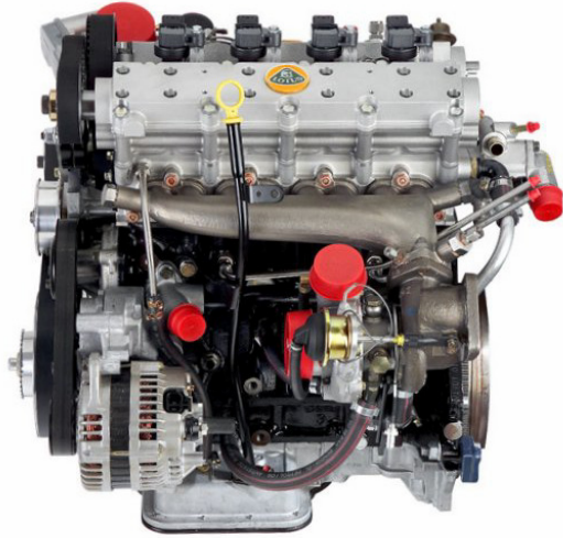
Fig. 4.3(b): Photograph of left hand (exhaust) side of Nomad research engine in the form used for initial turboexpansion testing reported by Turner et al. (2005a). (Photograph courtesy Lotus Engineering)
