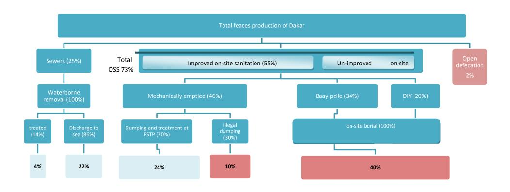
Figure 7-2: Sanitation cityscape of faecal sludge flows
