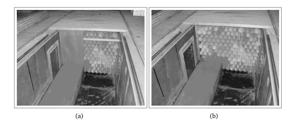
Figure 3.8: Arrangement at flume inlet (a) with board and (b) without board
