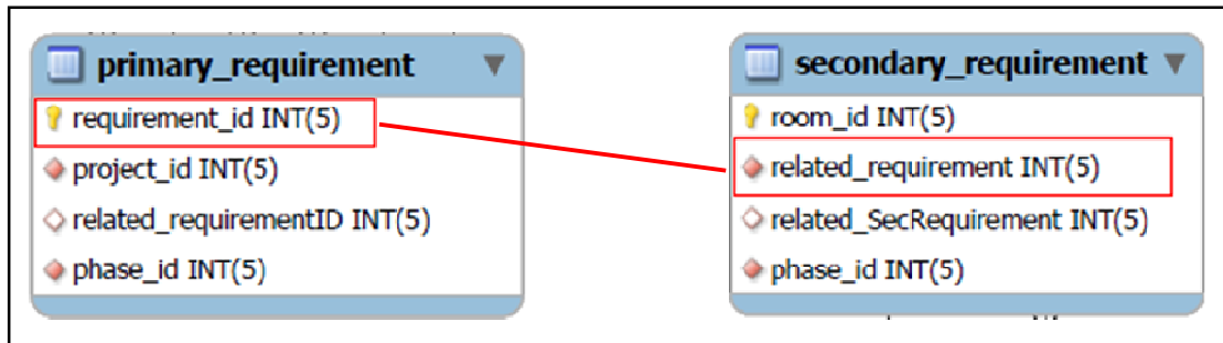
Figure 8.6: Dependency link between primary requirements and secondary requirements
