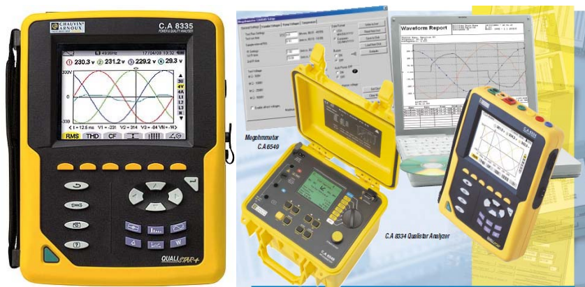
Figure 8.3: The Chauvin Arnoux C.A 8335 Qualistar Plus and the graphical outputs when used with the Dataviewer Pro
