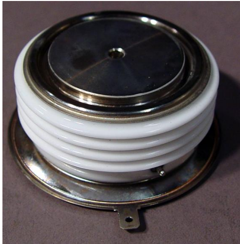
(c) Press-pack (or hockey-puck) thyristor construction
