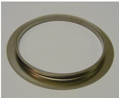
Figure 7.30: Photo of a nickel-plated flange used in the development of the 50 mm prototype
