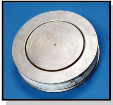
Figure 1.5: Photo of a 125 mm hockey-puck thyristor, sourced from Woodhouse, 2007b
