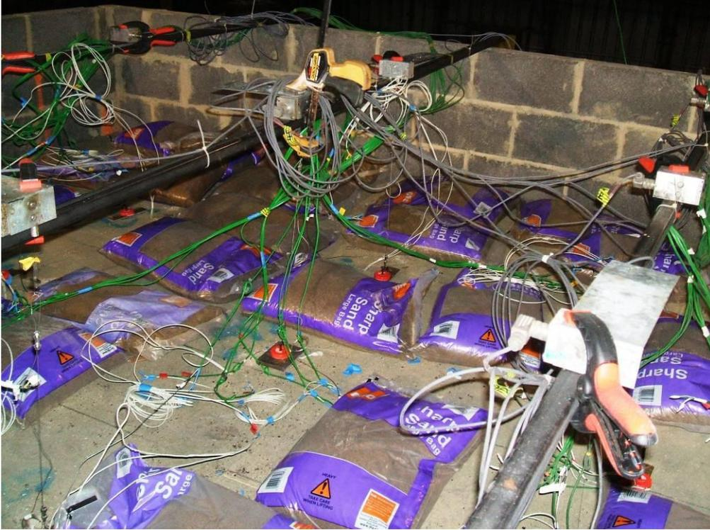
**Figure A.7. Floor plate with loading**
