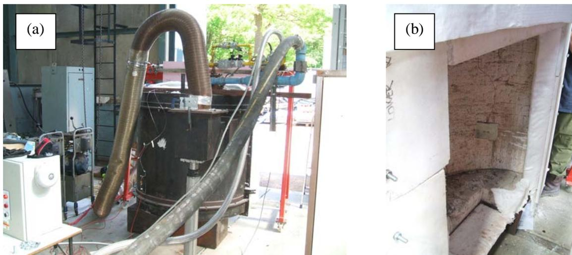
Figure 3.1 (a) External view of barrel furnace (b) Open side of the furnace
