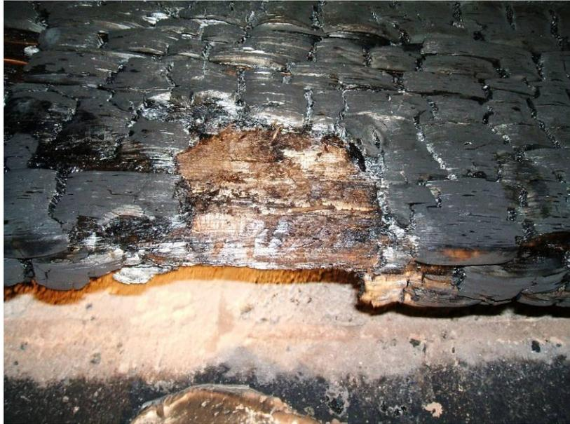
**Figure A.13. Depth of char on joist 2**
