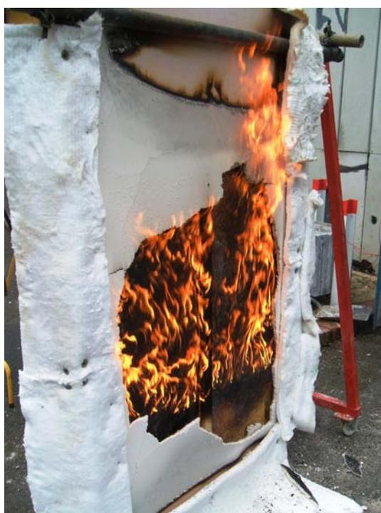
**Figure 4.11** Combustion of the fire side SIP OSB veneer
