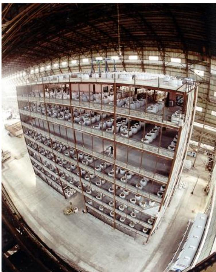
Figure 2.1 Steel building Cardington fire experiments
