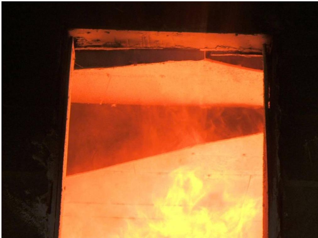
**Figure A.20. Evidence of plasterboard break away on ceiling, Test 3**
