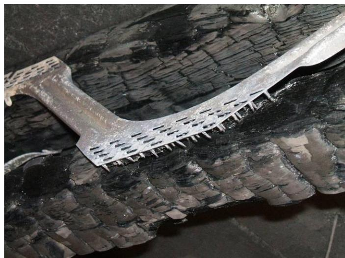
**Figure A.23- Tearing out of steel web elements**
