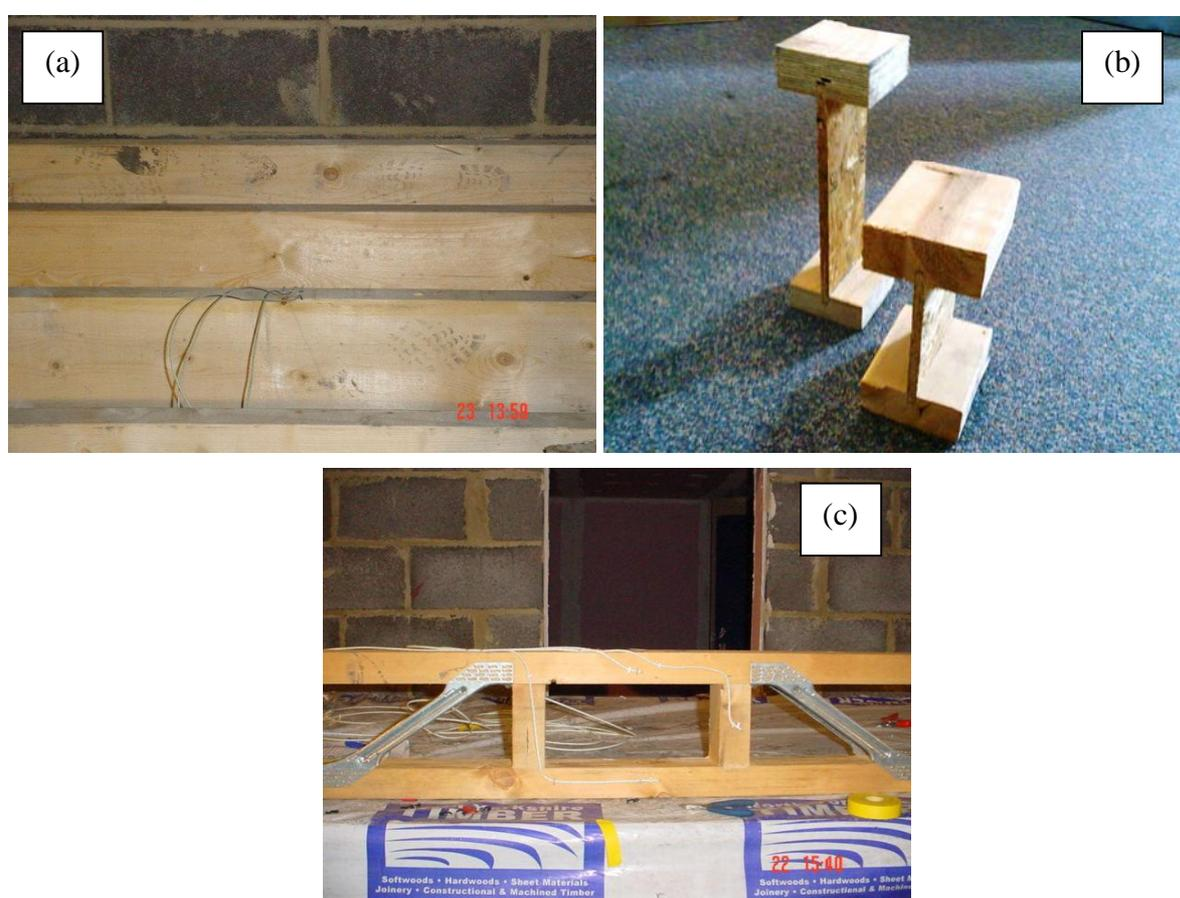
**Figure 4.1 Images of the joist systems tested (a) Solid joist (b) I-Joist (c) Steel truss web joist**
