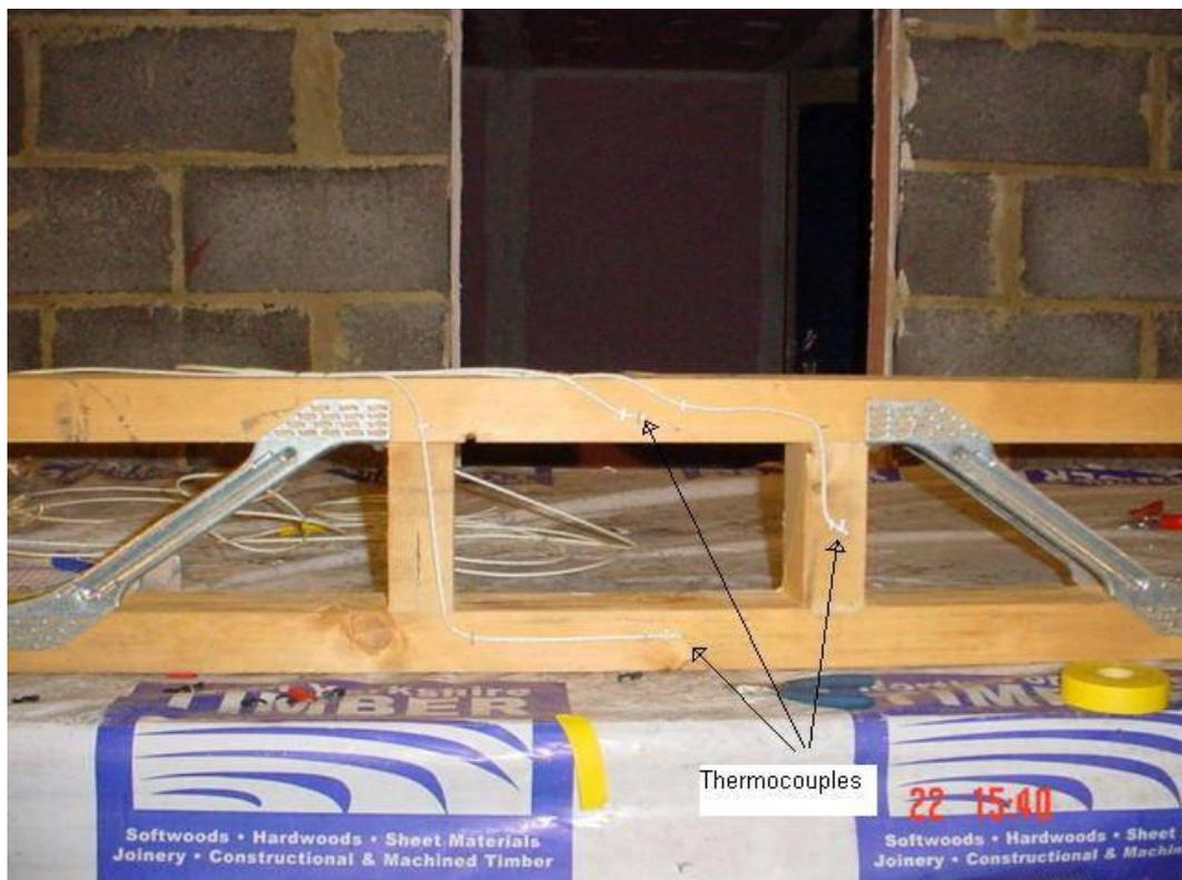
**Figure A.5. Joist instrumented with thermocouples (shown with arrows)**
