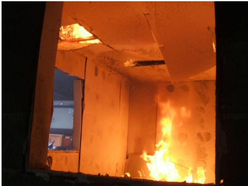
**Figure A.11. Fall away of plasterboard layers on ceiling**
