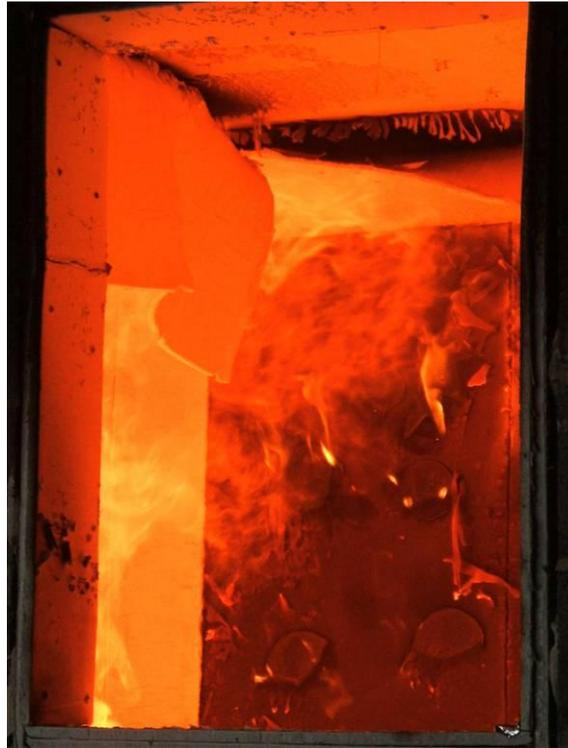
**Figure A.16. Fall off of first layer of plasterboard in Test 2**
