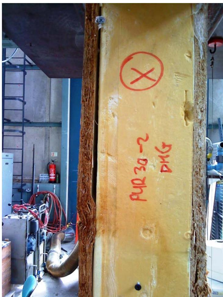
**Figure 4.3 Failure mode in an isolated SIP at ambient temperature**
