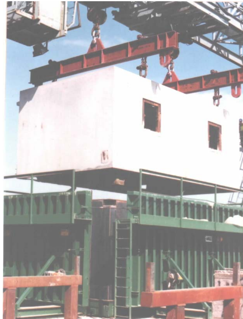
Figure 2 Modular building - Manufacture of precast concrete units for Fazakerley Prison Courtesy of Precast Cellular Structures Ltd.
