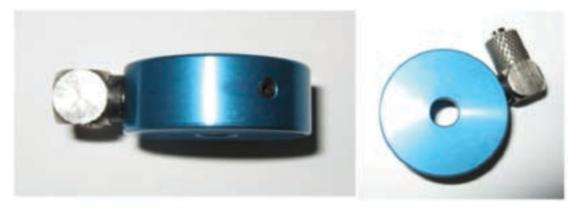
Figure 67: Nozzle used for processing very thick materials and 3D objects
