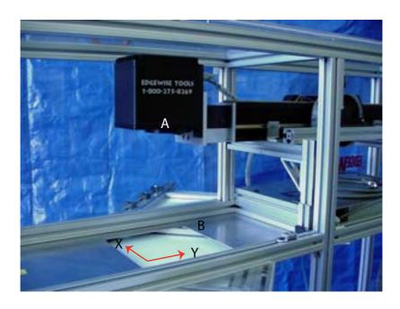
Figure 51: Galvanometer laser system. The beam is directed by mirrors from A on the work bed B and is able to process in both the x- and y- directions. The whole system is contained in a housing. (Edgewise Tools, 2011)
