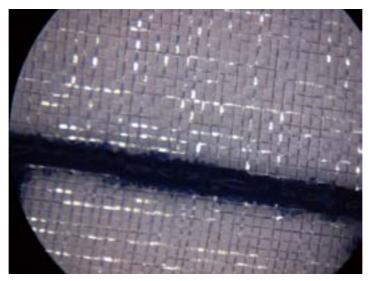
Figure 296: Sintered blue embossing powder on nylon organza, detail (underneath view)
