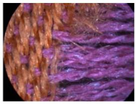
Figure 207: Silk twill with top surface removed by laser marking. (left) Pink warp threads intact (20/5/3/0.2). Detail (right)
