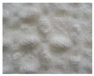
Figure 247: Plain weave, 5mm circles, 100mm apart - raised surfaces on back and front are similar
