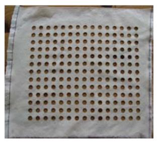
Figure 258: 10mm holes spaced 10mm apart
