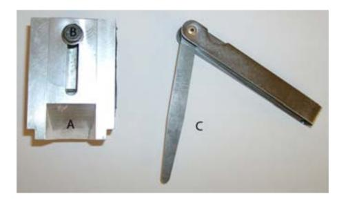
Figure 267: Powder spreader (M. Gibson) left. The centre section (A) may be adjusted up and down to change the thickness of the layer being spread by turning the screw (B). The feeler gauge (C right) is used to set the height of the spreader to the correct setting.
