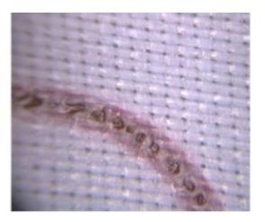
Figure 282: Sample C7 (detail) Four layers sintered onto paper nylon using a 50/50 mix of polyamide and embossing powders, top view (left), underneath view (right)
