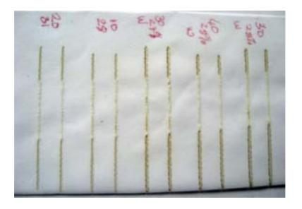
Figure 269: Sample of sintered lines with varying powers and speeds. Powder was spread along the centre of this sample.
