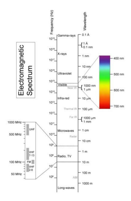
Figure 44: Diagram showing electromagnetic spectrum. The right-hand columns dives the wavelengths corresponding to wave in the central column.
