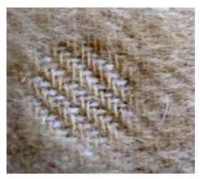
Figure 204: Camel/white twill with pile removed to reveal weave structure (15/5/5/0.2)
