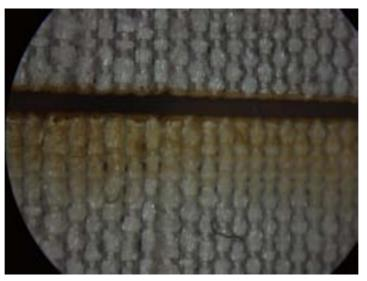
Figure 53: Silk dupion processed on flying optic system with compressed air. Charring is blown to one side of cut
