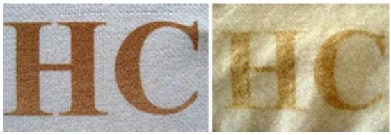
Figure 230: HC text pre finishing (left), HC text after two finishing washes (right)
