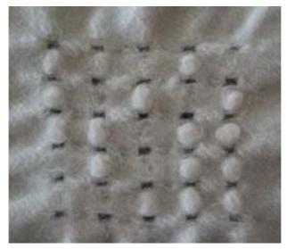
Figure 244: Raised areas produced by ovals (sample 4). Compared with Figure 243, it can be seen than these produce a more pronounced raised area in one direction.
