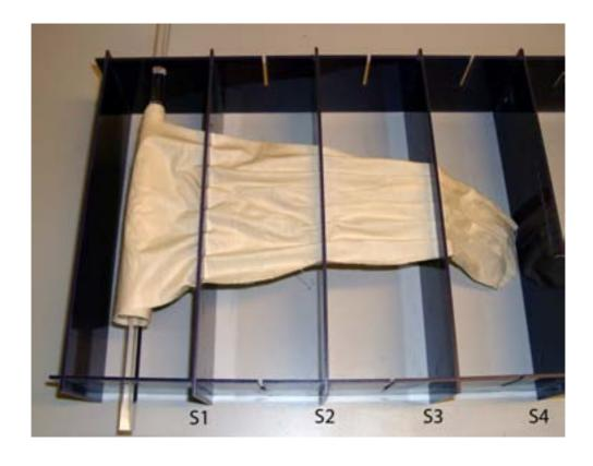
Figure 109: Fabric from the cylinder is passing through the cut-outs on the slots S1-S3 and is gradually being pleated.
