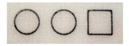
Figure 294: Linen substrate, blue embossing powder, 2.8W, 9mm/s, underneath views showing leaching of melted powder.
