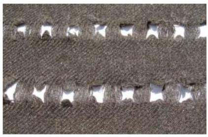
Figure 215: 32 threads removed, 1cm cuts 1cm apart in middle of space, position of cuts even on each row (5/15/5)
