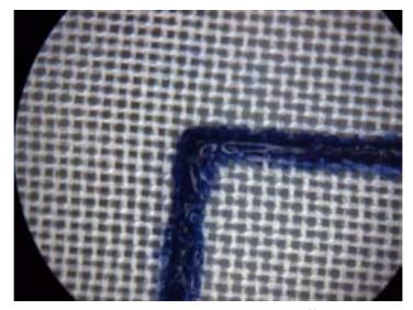
Figure 295: Sintered blue embossing powder on nylon chiffon, detail (underneath view)
