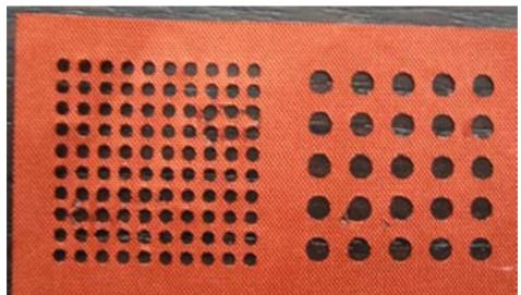
Figure 84: Polyester processed with the lowest power/highest speed parameters.
