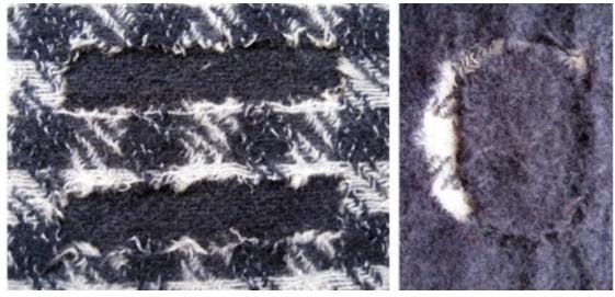
Figure 208: Double cloth with bands of top the checked layer removed to show the navy blue under layer (10/6/3/.2), (left), : 'C' etched on reverse of double cloth - insufficent detail and frayed edge (10/8/3/0.2 x 2), (right)
