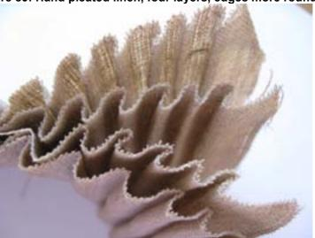
Figure 90: Hand pleated linen, four layers, internal folds are more sharply creased
