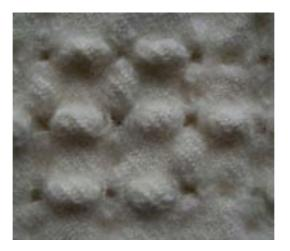
Figure 248: 2/2 twill, 5mm circles, 10mm apart – raised surfaces on back and front are similar
