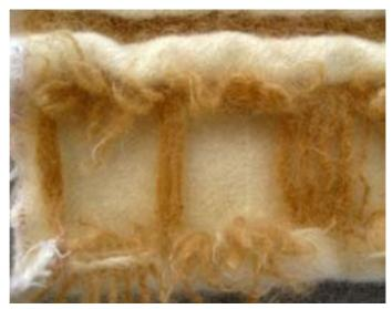
Figure 264:The same in Figure 260 post finishing. The fabric ground has contracted and the loose floats have felted forming pockets.
