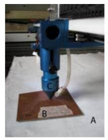
Figure 64: Work area flying optics system. Material (A) is placed on the work bed. A plated (B) of known thickness is placed under nozzle (C) and the gap adjusted.
