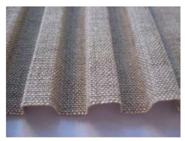
Figure 101: Folded linen produced using the slatted boards
