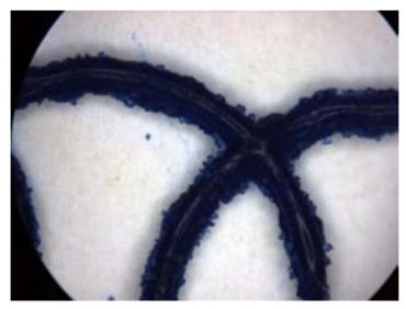
Figure 302: Blue embossing powder sintered onto Aquasol which has been dissolved. Unmelted grains of powder may be seen attached to the sintered forms, giving a rough surface
