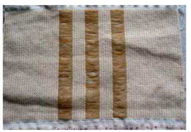
Figure 261: Warp 2/08 Ground snow, caramac floats, bound in with two warps
