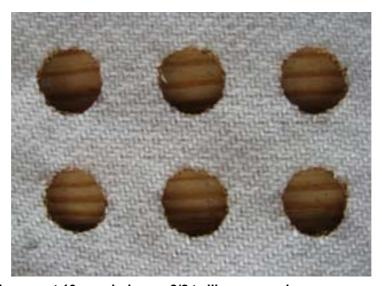
Figure 233: Laser cut 10mm circles on 2/2 twill, snow cashmere warp and weft, detail
