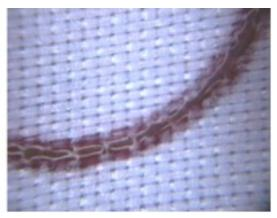
Figure 277: Sample C4 (detail), red embossing powder, paper nylon, 2.8W, 9mm/s, top view(left), underneath view (right)
