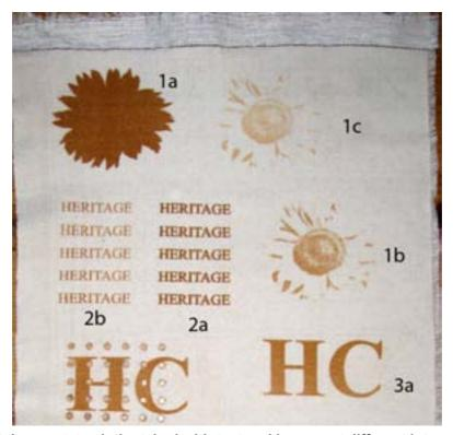
Figure 224: Loom state cloth etched with text and images at different intensities, prefinishing
