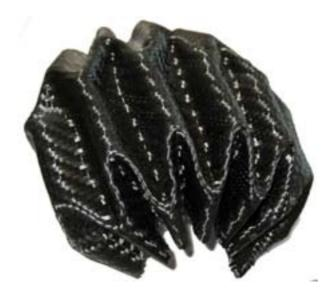
Figure 193: Rigid carbon fibre structure formed from the template in Figure 189.
