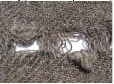
Figure 214: Detail from figure above showing matted fringe on alternate side of gap
