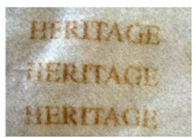
Figure 229: Fine text after one finishing wash. (left) The block of text on the left (light etching) is already very faint. Fine text after two finishing washes. (right) Images show the right most block from Figure 228 (etched with medium settings)
