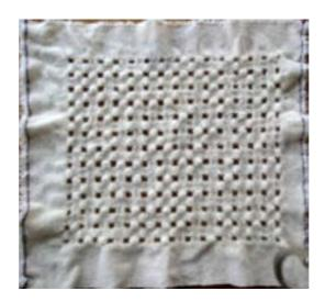
Figure 235: Fabric after two finishing washes. Bobbles have formed resulting in a three-dimensional surface
