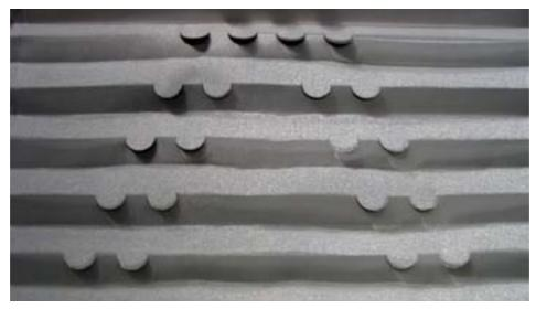
Figure 126: Laser cut polyester organza shown attached to the bottom template, after steaming
