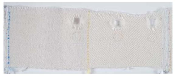
Figure 219: Warp 1 showing cutting and marking tests. Photo K. Walton
