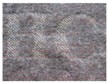
Figure 205: Grey pile removed to reveal twill structure (15/5/5/0.2)
