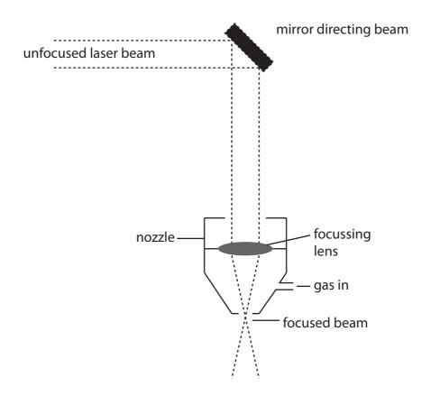
Figure 43: Diagram showing how a laser beam is directed, using a mirror, to a lens which focuses the beam to a spot. The lens is housed inside the nozzle, which has an air intake on the side for an assist gas
