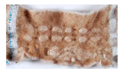
Figure 239: The sample cuts in Figure 238. Large holes cause the fabric to become unstable. Small holes and squares produce three-dimensionality. Photo K. Walton
