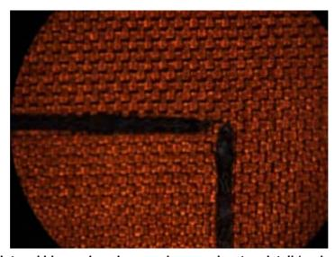
Figure 299: Sintered blue embossing powder on polyester, detail (underneath view)
