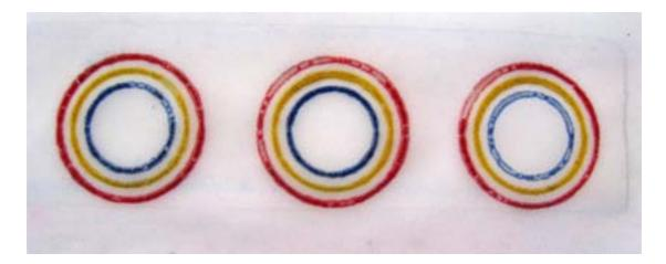
Figure 283: Red (20mm circle), yellow (16mm circle) and blue (12mm circle) embossing powders sintered on paper nylon, 2 layers.
