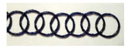
Figure 301: Blue embossing powder sintered onto Aquasol which has been dissolved
