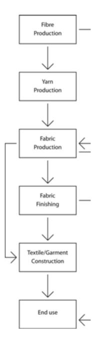
Figure 1: Production stages in the manufacture of textiles
