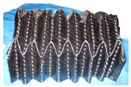
Figure 192: Rigid carbon fibre structure formed from the template in Figure 189
