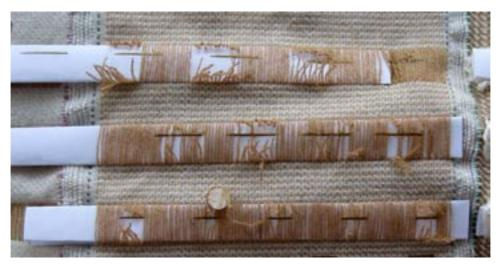
Figure 262: Detail of Figure 261 after laser cutting . Paper inserted prior to cutting to protect the fabric underneath.
