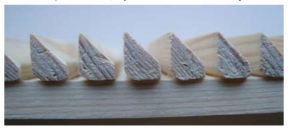
Figure 102: Board with slats that have a zigzag profile
