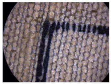
Figure 297: Sintered blue embossing powder on silk dupion, detail (underneath view)
