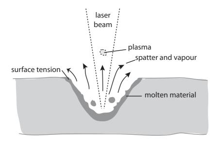
Figure 46 : Diagram showing molten material and vapour at the beam interface during laser processing
