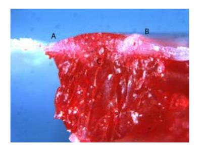
Figure 278: Cross section of sample C4 (fabric at top, sintered layers below.
