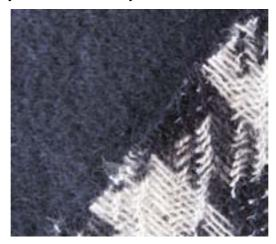
Figure 197: Double cloth (cashmere), checked layer interwoven with plain layer. The weave structure of the two layers is very different
