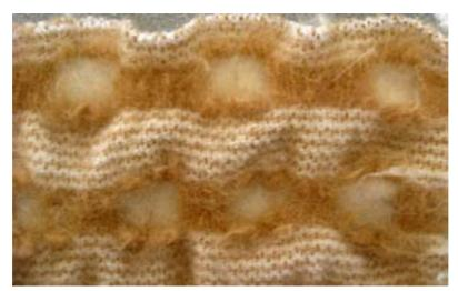
Figure 263: Post finishing, the fabric ground and the remaining floats shrink resulting in pockets
