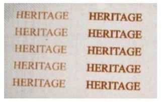
Figure 228: Fine text after etching, light and medium settings
