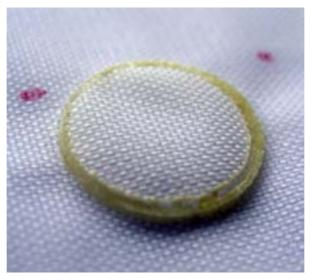
Figure 286: Three- dimensional sintered structure, polyamide powder, paper nylon top and bottom, 10mm circle 4 layers, option a.
