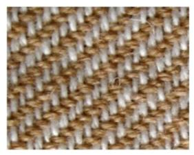
Figure 196: 2/2 Twill, snow cashmere warp, caramac weft, even proportions of colour on both sides of the fabric
