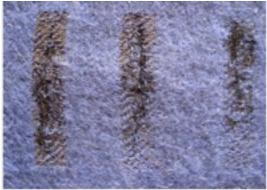
Figure 203: Double faced plain weave with laser marking (10/6/2/0.2) Blue pile has been removed and fabric is stable. (left) Sufficient blue pile has been removed to reveal the black under layer but has damaged the fabric structure (right)
