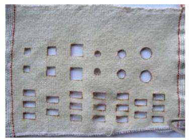
Figure 238: A sample looking at the effect of cut-out shape. Squares (5mm, 7.5mm, 10mm) Circles (5mm, 7.5mm, 10mm) Rectangles 10mm x 5mm
