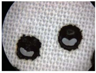
Figure 307: Cut holes sintered with black embossing powder and partially filled
