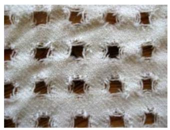
Figure 234: Fabric after one finishing wash, detail. Circles have started to form squares
