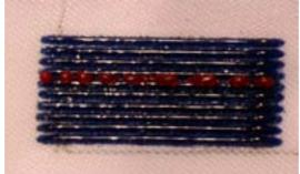
Figure 290: Sample B8. 2.8W, 10mm/s. tracks 1mm apart. Layers 0.25, 0.4, 0.6, 0.9 Blue, 1mm red
