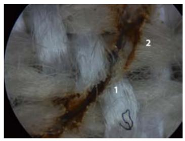
Figure 198: Laser cut polyester/cashmere cloth. Horizontal thread (2) is cashmere showing charring. Vertical polyester thread (1) shows melting and no charring
