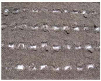
Figure 213: 16 threads removed, 1cm cuts 1 cm apart, alternately close to top edge then bottom edge, position of cuts in same place on each row (5/15/5)
