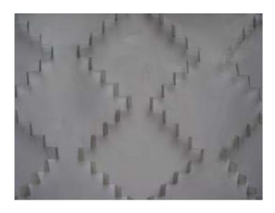
Figure 188: Stainless steel formed into a three-dimensional surface with laser assited template pleating
