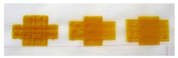
Figure 292: Yellow embossing powders on paper nylon, tracks 0.6mm, 0.8mm and 1mm apart, layers 0.25mm horizontal, 0.4mm vertical, 0.6mm horizontal, 0.9mm vertical
