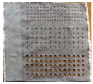
Figure 242: 7.5mm semi circles, 10mm crosses, 10mm circles
