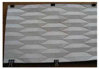
Figure 191: Carbon fibre sandwiched between two pre-folded templates. This will be refolded prior to heat setting.
