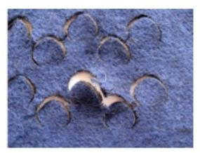
Figure 202: Laser cut (5/20/3) and pressed double faced plain weave – blue on one face and black on the other (left), sample after post processing. (right) Edges show fraying and the fabric has disintegrated in parts
