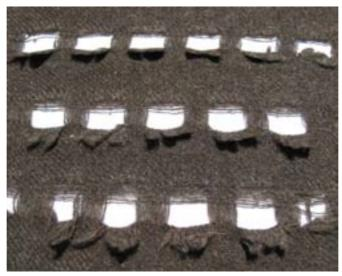
Figure 211: 16 threads removed, 2cm cuts 1cm apart, close to top edge, position of cuts alternates on each row (5/15/5)
