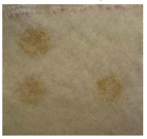
Figure 221: 100% cashmere etched. Pile raised post processing and charring mark integrated within fabric
