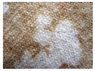
Figure 232: Detail of etching in Figure 231 showing the marked areas fully integrated in the fabric with no obvious fibre degradation.
