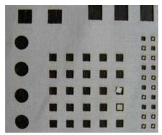
Figure 68: Cotton processed with beam set to correct focus height (1mm)
