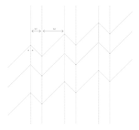
Figure 183: Origami design, uneven pleat spacing
