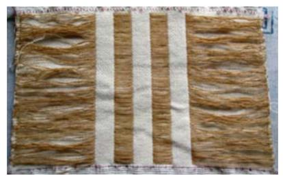
Figure 260: Warp 2/09 Ground snow, caramac floats, loosely attached to selvedge
