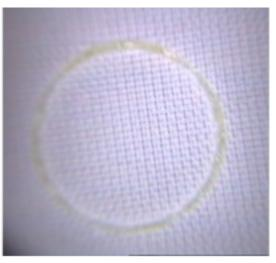
Figure 271: 10mm circle, 4 layers on sintered polyamide powder on paper nylon, Sample 10 :0.25mm/ 0.38mm/ 0.63mm/ 0.9mm, 6mm/s, 2.8W. Top view, (left), underneath view (right)
