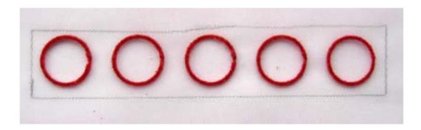
Figure 276: Red embossing powder sintered on paper nylon, 10mm circles
