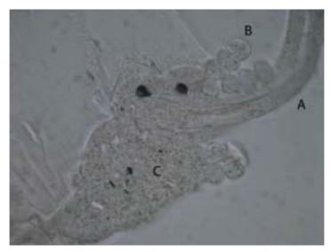
Figure 274: Cross section of sample 10 showing warp and weft threads (A, B) and area were textile substrate and polymer powders have fused
