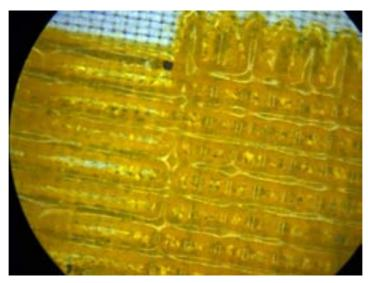
Figure 293:Yellow embossing powders sintered on paper nylon (detail of 1mm tracks in previous image), alternate layers of tracks at right angles, detail. Ridged surface may be seen
