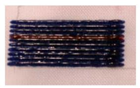
Figure 291: Sample B9. 2.8W, 10mm/s layer 1, 9mm/s layers 2-6. tracks 1mm apart. Layers 0.25, 0.4, 0.6, 0.9 blue, 1mm red
