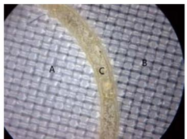
Figure 288: Two layers A (top) and B (bottom) joined by sintered weld (C), underneath view.
