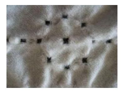
Figure 246: 100mm circle cut-outs placed in a circle layout (sample 5). The spacing of the cut-outs is too far apart to generate much three-dimensionality.
