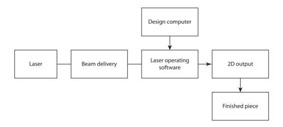
Figure 48 : Diagram showing a textile laser processing system
