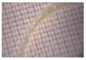
Figure 272: Detail of sample 10 in Figure 271. Top view, (left) shows loose unmelted powder attached to the sintered circle. Underneath view (right) showing the fused weld.
