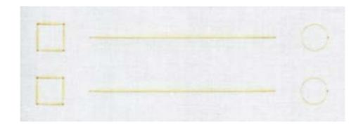
Figure 75: Cotton showing uneven marking, the circles are much lighter that the lines and squares
