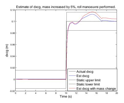
Figure 101: Robustness test, roll, dxcg, mass increased by 5%
