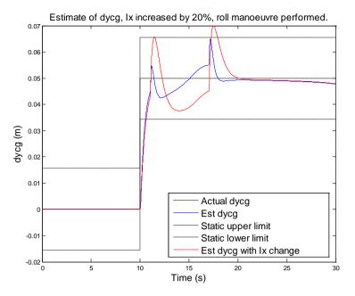
Figure 107: Robustness test, roll, dycg, Ix increased by 20%
