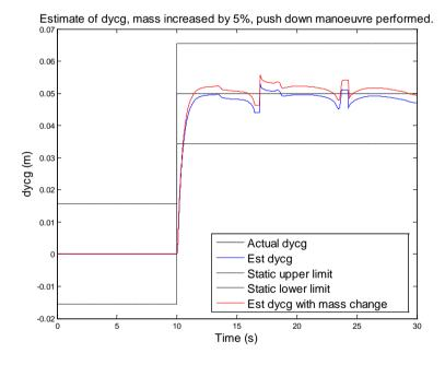
Figure 106: Robustness test, push down, dycg, mass increased by 5%
