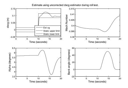
Figure 91: Uncorrected dxcg estimator. Roll test.
