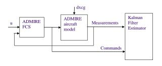
Fig. 1. Aircraft model and estimator.
