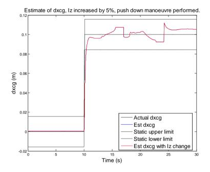
Figure 96: Robustness test, push down, dxcg, Iz increased by 5%
