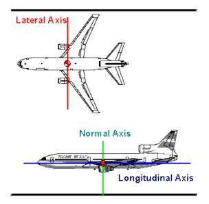
Figure 1. Aircraft axes through cg (Geistware, 2010).
