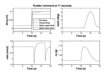
**Figure 49: Lateral acceleration test**
