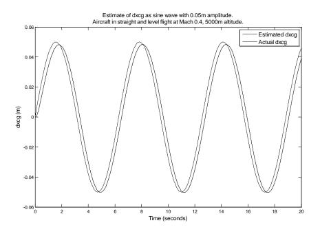
Figure 24: Estimate of sine wave longitudinal cg shift. No measurement noise.
