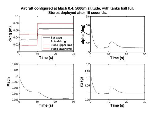
Figure 75: CG estimate with store deployment. Fuel tanks half full.
