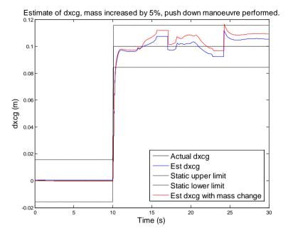
Figure 97: Robustness test, push down, dxcg, mass increased by 5%
