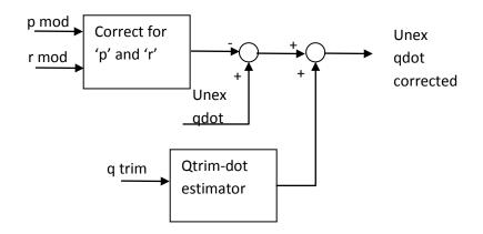
Figure 45: Longitudinal cg estimator corrections
