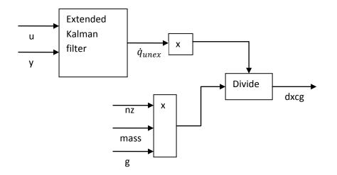
Figure 82: Structure of extended Kalman filter for longitudinal cg estimator
