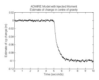
Fig. 8. CG Estimate using linear ADMIRE model and injected moment.
