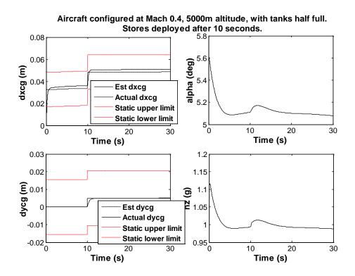
Figure 76: CG estimate with store deployment. Fuel tanks half full.
