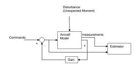
Fig. 1. Aircraft Model with model-based Estimator.
