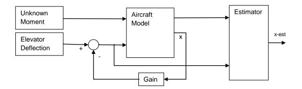
**Figure 9: Aircraft model with estimator**
