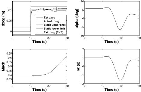
Full push down at 15.5 seconds over 5 seconds then return to zero over 5 seconds.
