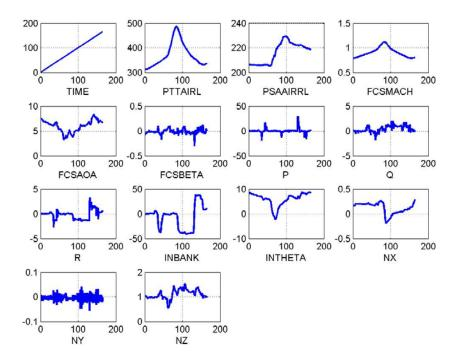
Appendix D – Flight test measurement noise data
