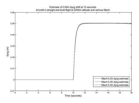
Figure 32: Estimate of lateral cg change. Aircraft at Mach 0.25, 0.35 and 0.45 at 2000m altitude.
