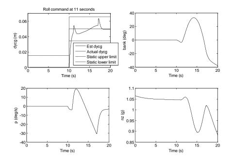
Figure 60 : Roll test.
