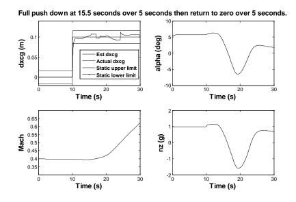
Figure 51: Pitch stick push down test
