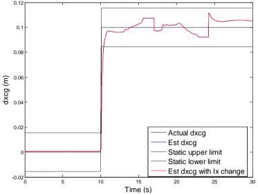
Estimate of dxcg with Ix increased by 20%, and push down manoeuvre performed.
