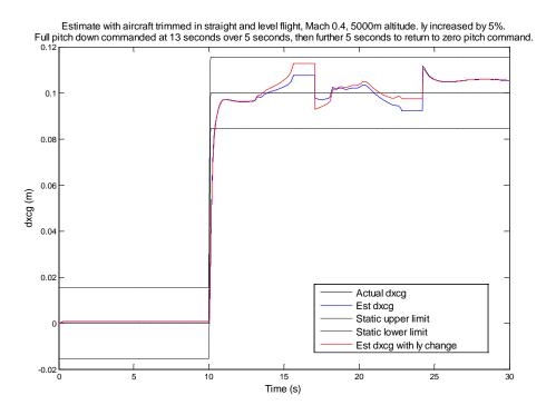
Figure 67: Estimate of longitudinal cg change of 0.1m. Aircraft in push down manoeuvre. Iy increased by 5%.
