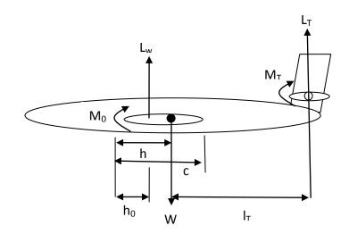
Figure 8: Trimmed aircraft in level flight
