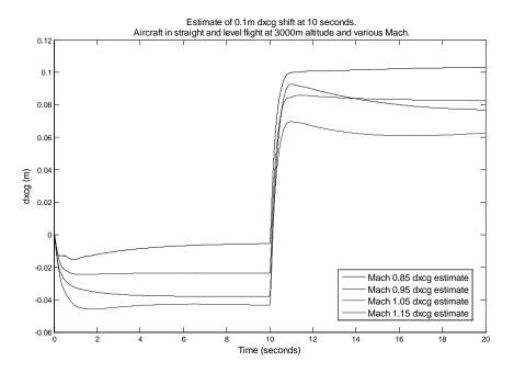
Figure 27: Estimate of longitudinal cg change at Mach 0.85, 0.95, 1.05 and 1.15 at 3000m altitude. No noise added.
