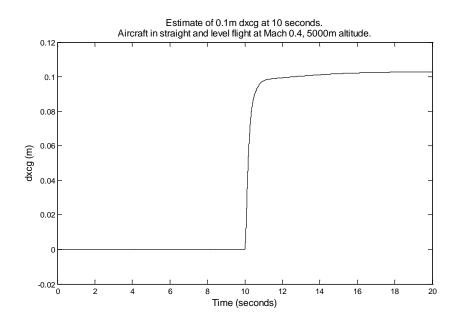
Figure 22: Estimate of 0.1m change in longitudinal cg. No measurement noise.
