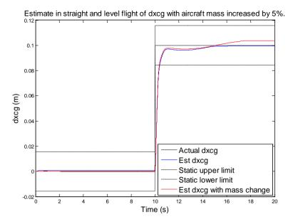
Figure 93: Robustness test, straight-level, dxcg, mass increased by 5%
