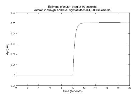
Figure 30: Estimate of 0.05m change in lateral cg. No measurement noise.
