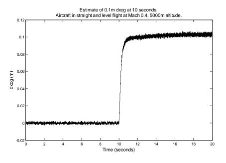
Figure 21: Estimate of 0.1m change in longitudinal cg. Aircraft trimmed at Mach 0.4, 5000m altitude.
