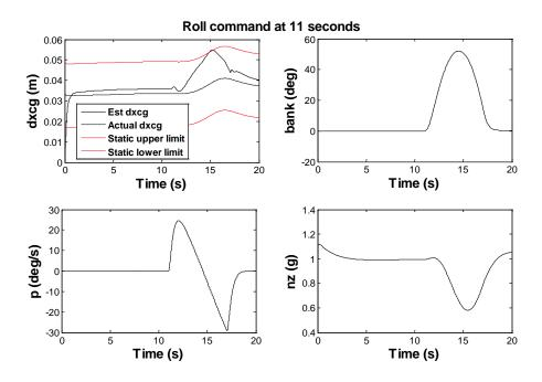
**Figure 72: CG estimate during roll test using BAE cg modifier. Fuel tanks half full.** The rudder test (Figure 71) generated virtually no change in dxcg, and the estimate stays accurate.
