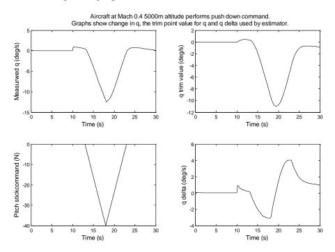
Figure 46: Effect of change in AoA on the measured 'q' and delta 'q' used by the cg estimator.
