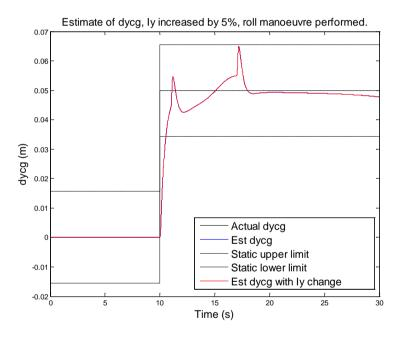
Figure 108: Robustness test, roll, dycg, Iy increased by 5%
