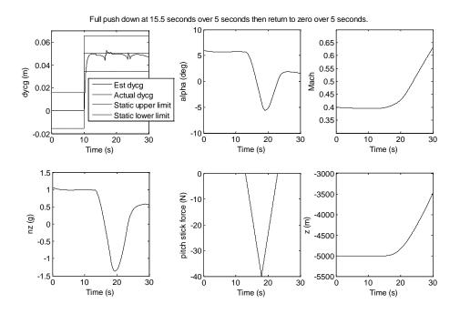
Figure 61: Push down test.
