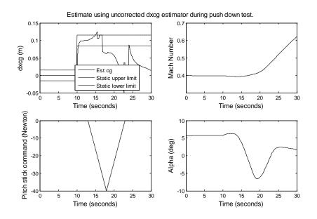
Figure 90: Uncorrected dxcg estimator. Push down test.
