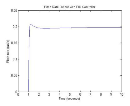
Figure 15: Phantom model with PID controller – pitch rate output
