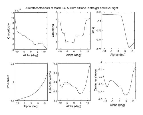
Figure 42: ADMIRE aircraft pitching moment coefficients at various AoA
