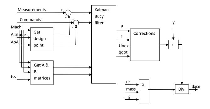
Figure 44: Longitudinal cg estimator structure
