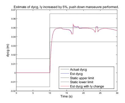
Figure 104: Robustness test, push down, dycg, Iy increased by 5%
