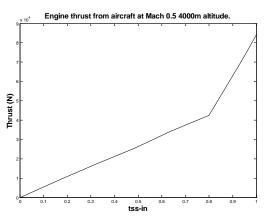
Fig. 4. Engine thrust output from tss command, aircraft at Mach 0.5 and 4000m altitude.
