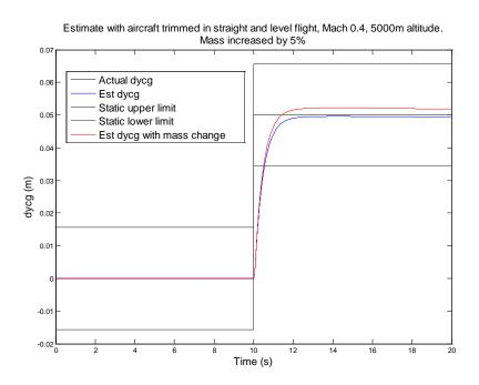
Figure 68: Estimate of 0.05m lateral cg change. Mass increased by 5%.
