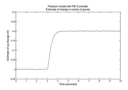
Figure 17: CG estimate for Phantom model with changing pitch rate
