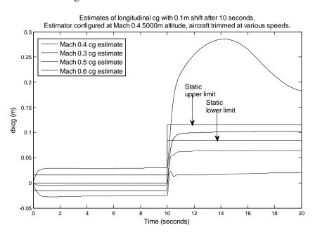
Figure 35: Estimate of change in longitudinal cg. Aircraft at various speeds, estimator configured for Mach 0.4 5000m altitude
