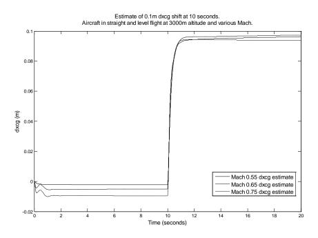
Figure 26: Estimate of longitudinal cg change at Mach 0.55, 0.65 and 0.75 at 3000m altitude. No noise added.
