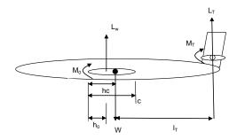
Fig. 3. Forces and Moments on Horizontal Trimmed Aircraft contained in [13].
