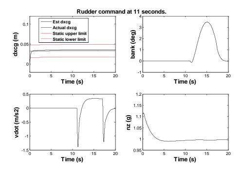
Figure 71: CG estimate during lateral acceleration using BAE cg modifier. Fuel tanks half full.
