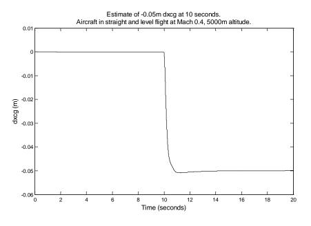
Figure 23: Estimate of -0.05m change in longitudinal cg. No measurement noise.
