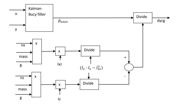
Figure 28: Structure of lateral cg estimator
