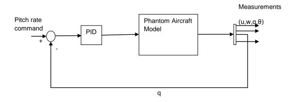
Figure 14: Phantom model with PID controller
