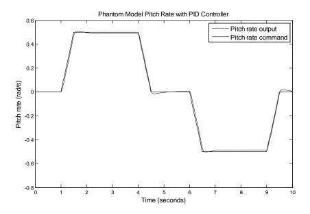
Figure 16: Phantom model with PID controller - pitch rate command and output
