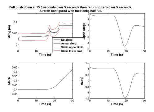
Figure 70: CG estimate during push down test using BAE cg modifier. Fuel tanks half full.
