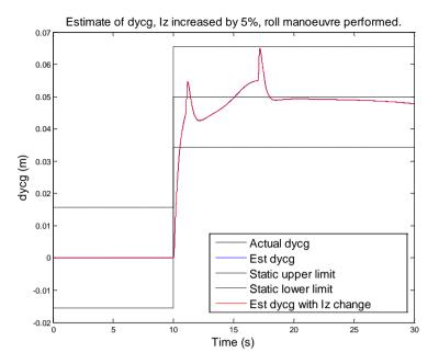
Figure 109: Robustness test, roll, dycg, Iz increased by 5%
