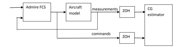
Figure 78: ADMIRE aircraft model with discrete cg estimator
