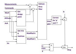
Fig. 3. CG estimator structure.
