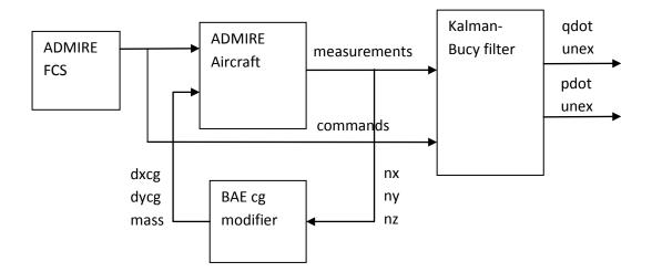
Figure 69: ADMIRE model with BAE cg modifier and estimator
