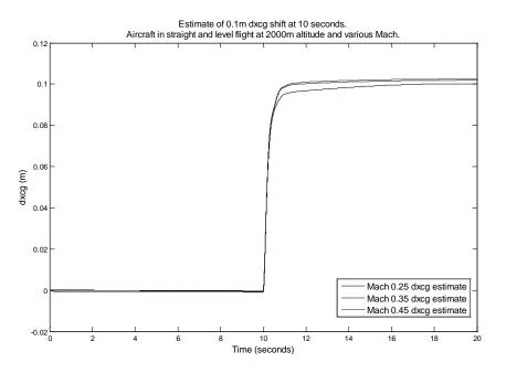
Figure 25: Estimate of longitudinal cg change at Mach 0.25, 0.35 and 0.45 at 2000m altitude. No noise added.
