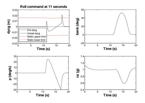
Figure 74: Lateral cg estimate during roll test using BAE cg modifier. Fuel tanks half full.
