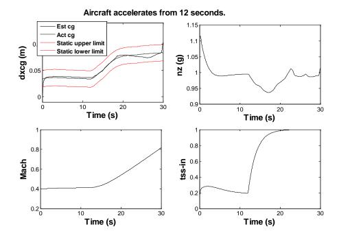
Figure 73: CG estimate during acceleration test using BAE cg modifier. Fuel tanks half full.
