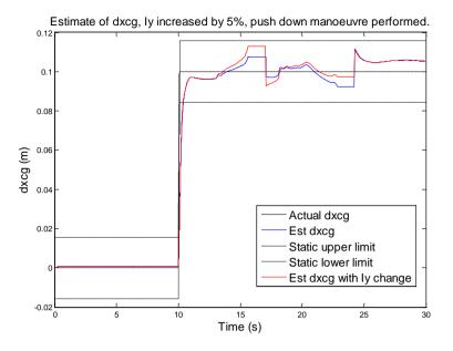
Figure 95: Robustness test, push down, dxcg, Iy increased by 5%
