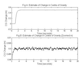
Fig. 4. Estimation of centre of gravity change from open-loop Phantom F4-C Aircraft Model
