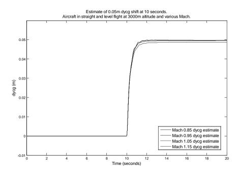
Figure 34: Estimate of lateral cg change. Aircraft at Mach 0.85, 0.95, 1.05 and 1.15, and at 3000m altitude.
