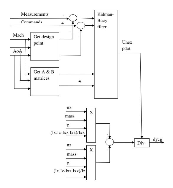
Figure 57: Lateral cg estimator structure
