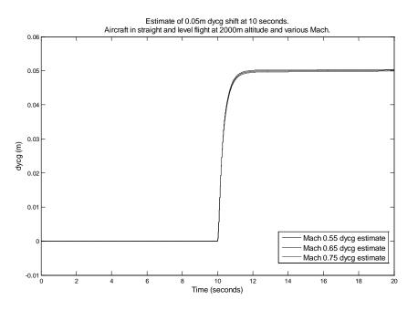
Figure 33: Estimate of lateral cg change. Aircraft at Mach 0.55, 0.65 and 0.75, at 3000m altitude.
