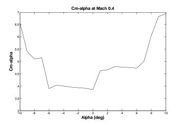
**Figure 41: Cm**<sub>α</sub> at Mach 0.4 and various angles of attack
