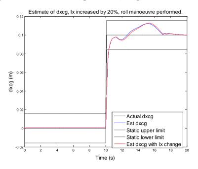
Figure 98: Robustness test, roll, dxcg, Ix increased by 20%
