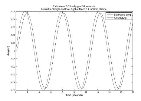
Figure 31: Estimate of sine wave lateral cg change.
