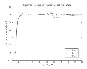
Fig. 5. Robustness tests of cg estimation on open-loop Phantom F4-C model..
