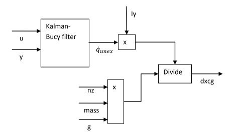
Figure 20: Structure of longitudinal cg estimator
