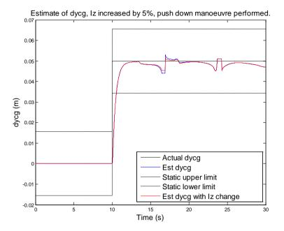
Figure 105: Robustness test, push down, dycg, Iz increased by 5%
