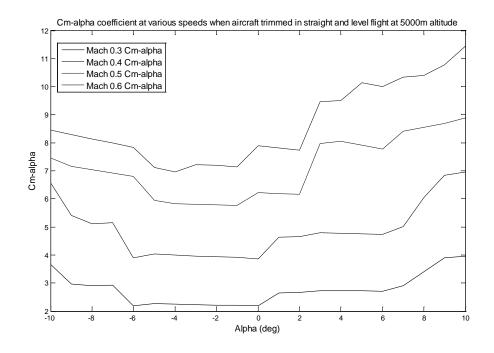
Figure 43: ADMIRE Cm<sub>a</sub> coefficient at various Mach and Aoa
