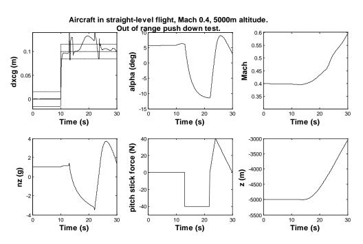
Figure 65: Out of range push down test.
