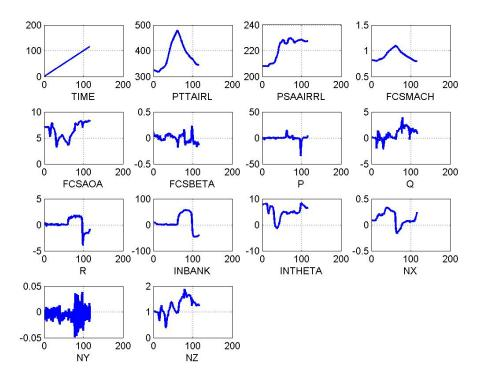
Figure 19: Sample flight test measurements used to obtain measurement noise
