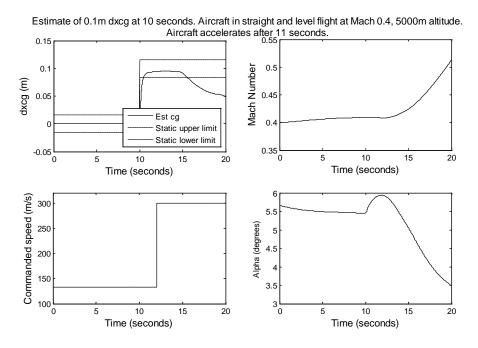
Figure 36: Uncorrected estimator. Acceleration test.
