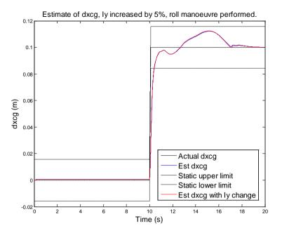
Figure 99: Robustness test, roll, dxcg, Iy increased by 5%
