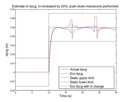
Figure 103: Robustness test, push down, dycg, Ix increased by 20%
