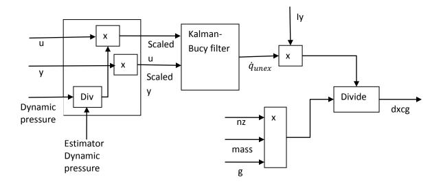
Figure 37: Longitudinal cg estimator using scaled inputs
