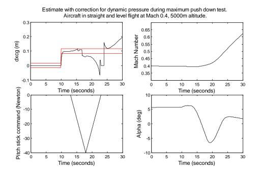
Figure 40: Longitudinal cg estimate during maximum push down manoeuvre. Estimator corrected for dynamic pressure and interpolated trim points.
