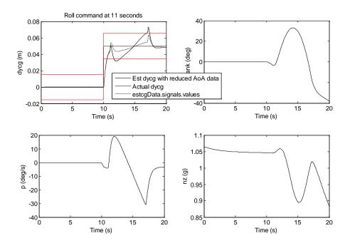
Figure 56: Estimate of lateral cg using different data point tables.
