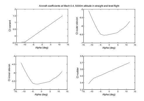
Figure 55: ADMIRE roll coefficients - commands.
