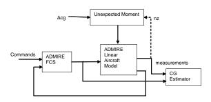
Fig. 7. Linear ADMIRE model with Injected Unexpected Moment.
