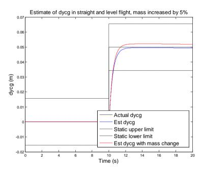
Figure 102: Robustness test, straight-level, dycg, mass increased by 5%
