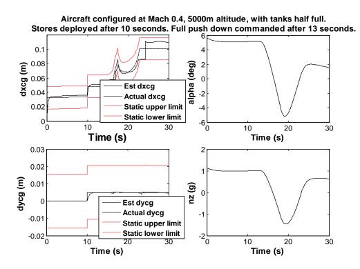
Figure 77: CG estimate with store deployment and max push down. Fuel tanks half full.
