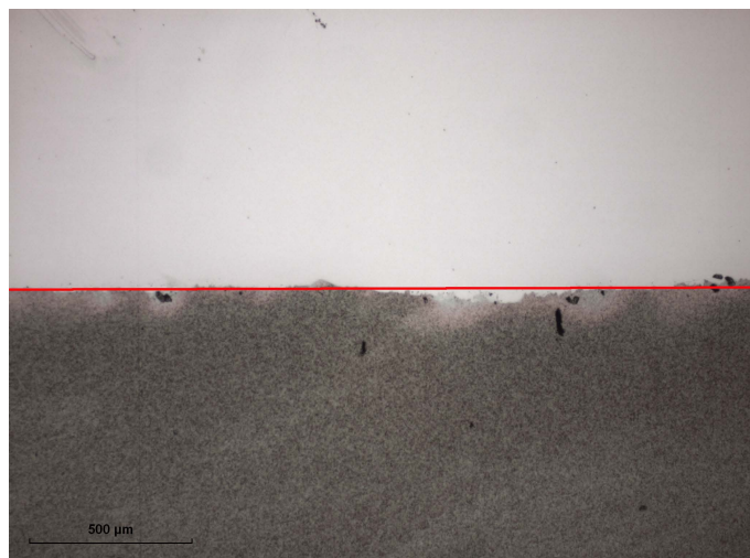
Figure 5.17: Optical microscope image showing the surface of an AZO film after being exposed to a 0.16\text{M HCl}_{(\text{aq})} solution for 60 seconds. Below the red line is the chemically treated part of the film which is highly etched by the acidic solution. This highlights the necessity to successfully protect the AZO surface.
