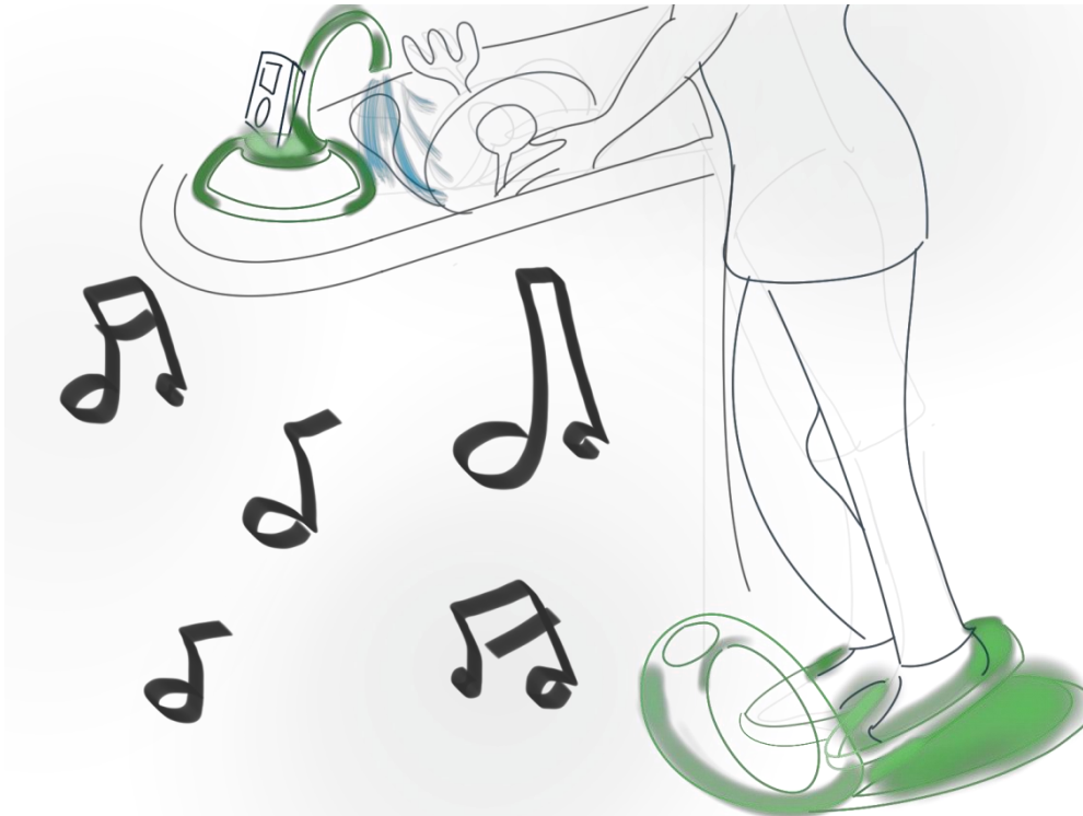
Figure 7-13, A case of a design output using punishment as a DfSB strategy (eco-spur), degenerating sound quality when using high quantities of water.
