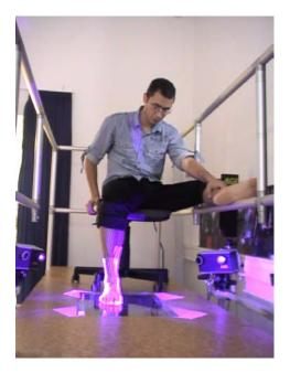
Figure 6.2. Participant having the foot scanned for the static design.
