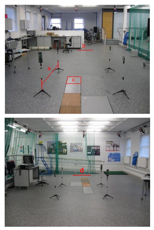
**Figure 5.7.** Views of the laboratory set up with the 10-m runway, electronic timing gates and Vicon system; (a: 2-metres distance between timing gates; b: start of the runway; c: the force platform used in the study; and d: end of runway).
