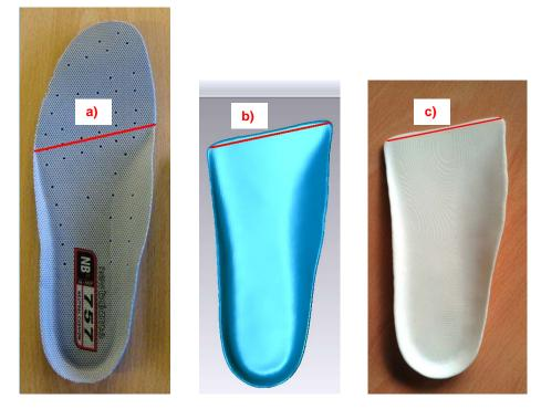
Figure 5.23. The control condition before the scan (left), during the design phase (centre) and after manufacturing (right). a) 96 mm; b) 94 mm; c) 93.2mm.
