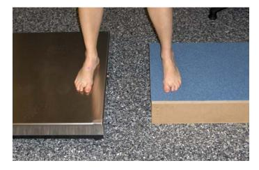
Figure 4.4. The set up showing scale (left) and a block (right) to facilitate taking anthropometric measurements.
