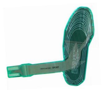
Figure 4.7. The Tekscan in-shoe plantar pressure sensor before trimming.
