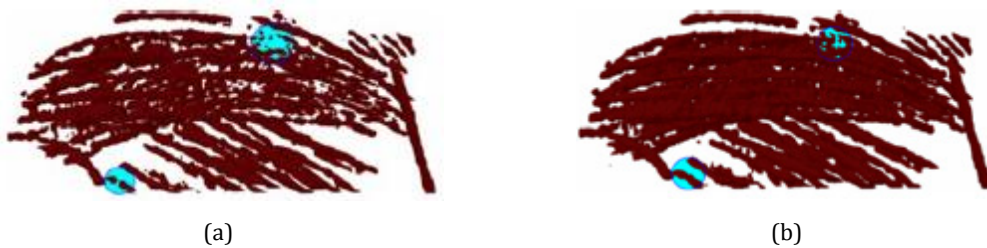
Figure 4.4 The effect of 5% change in threshold on fiber continuity. The highlighted parts are example of this discontinuity. (a) low threshold; (b) high threshold 194 .
