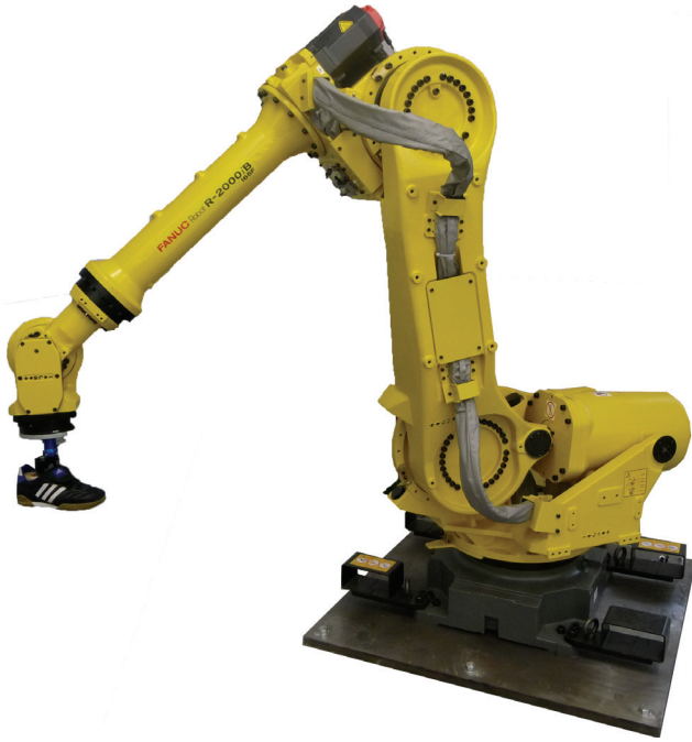
Fig. 1 The 6DOF Fanuc iRobot with shod prosthetic foot end effector attached
