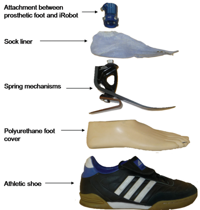
Fig. 2 Component parts of the shod prosthetic foot end effector
