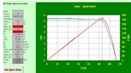
Figure 6 I-V characteristics for a Sanyo HIB 190Wp module measured in the SPIRE solar simulator.
