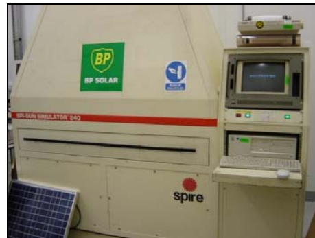
Figure 1 Picture of the CREST SPIRE 240 solar simulator (left) with its control unit (right).
