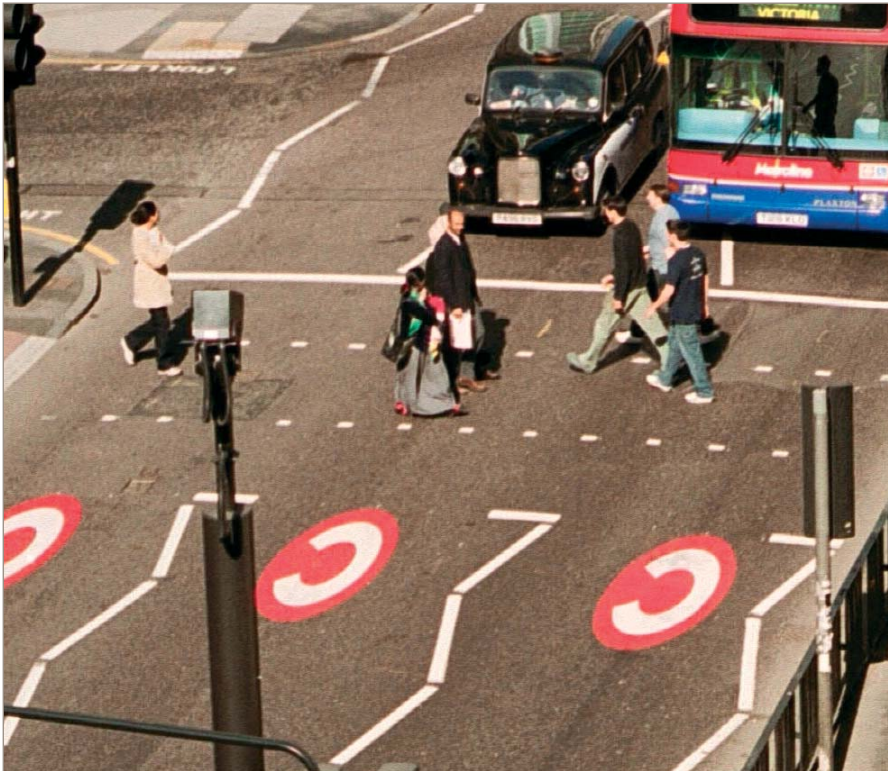
Fig. 3. Video cameras read the licence plates of vehicles entering the congestion-charging zone in central London, avoiding the need for in-vehicle equipment (courtesy of Marcus Enoch, www.transfoto.com)
