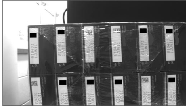
Figure 8. 2DBarcode Reader results on image under normal lighting conditions
