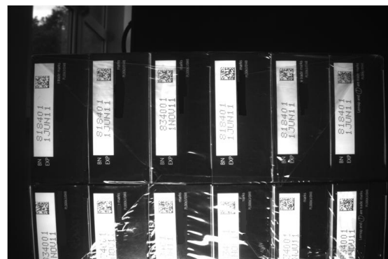
Figure 9(b). Image taken using Red LED backlight and red bandpass Filter
