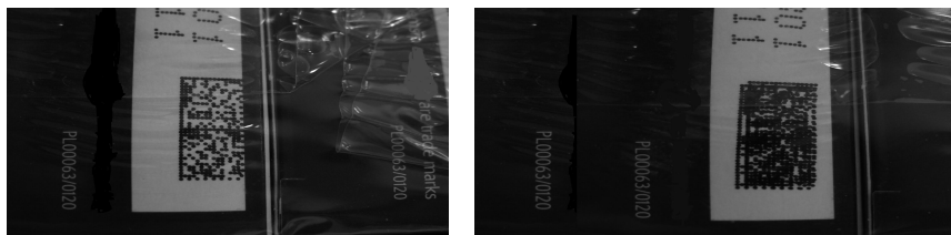
Figure 7. Non-decoded barcodes: Left – white background on one side is not present, Right – the print has been smudged.
